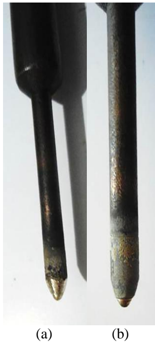
Fig. 10. Cathode tool wear: (a) Before machining, (b) After machining
