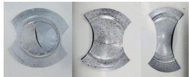
Fig. 8. Deformation of the test specimens after the Nakazima test
