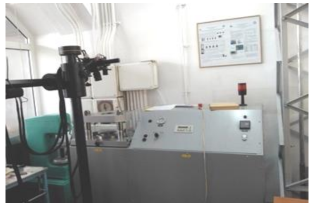
Fig. 2. Testing installation for Nakazima test
