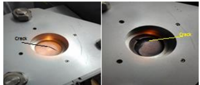
Fig. 7. Moment of crack occurred during the Nakazima test
