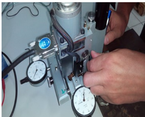
Fig. 4. Strain gauge bonded on the raceway of the bearing ring and its connection to indicator strains (a); drill centering support center of the strain gauge rosette (b)
