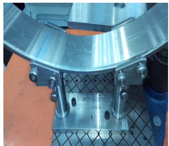
Fig. 2. Fixing the bearing ring in the test device
