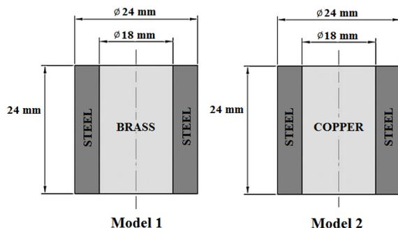
Fig.2. Design of Bimetallic Models
