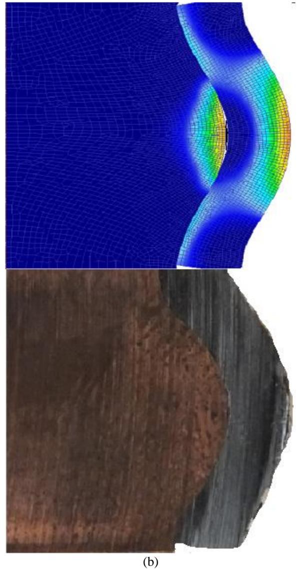
Fig.8. Comparison of FE simulation and experimental work after %40 reduction, (a) Model 1 (b) Model 2
