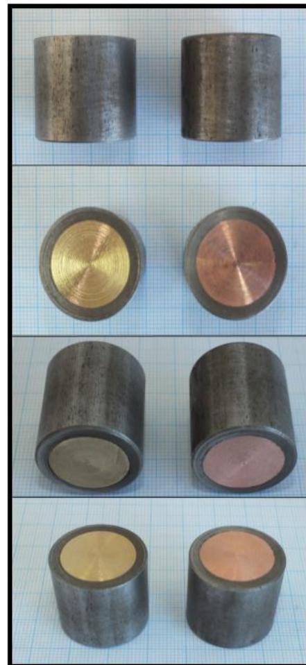
Fig.3. Obtained Bimetallic Parts
