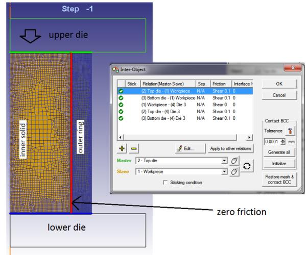
Fig.5. Meshed component and interactions
