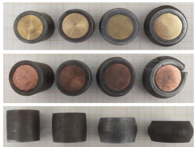
Fig.7. Deformations and barreling after %15, %30 and %40 reductions
