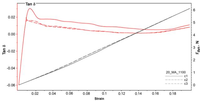
Fig. 6 Isothermal variations at  $T_2 = 533$  K of internal friction ( $\tan \delta$ ) and dynamic force ( $F_{dyn}$ ) of specimen 20\_MA\_1100, as a function of amplitude
