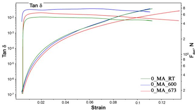
Fig. 7 Isothermal variations of average values of internal friction ( $\tan \delta$ ) and dynamic force ( $F_{dyn}$ ) of specimen 0\_MA\_700
