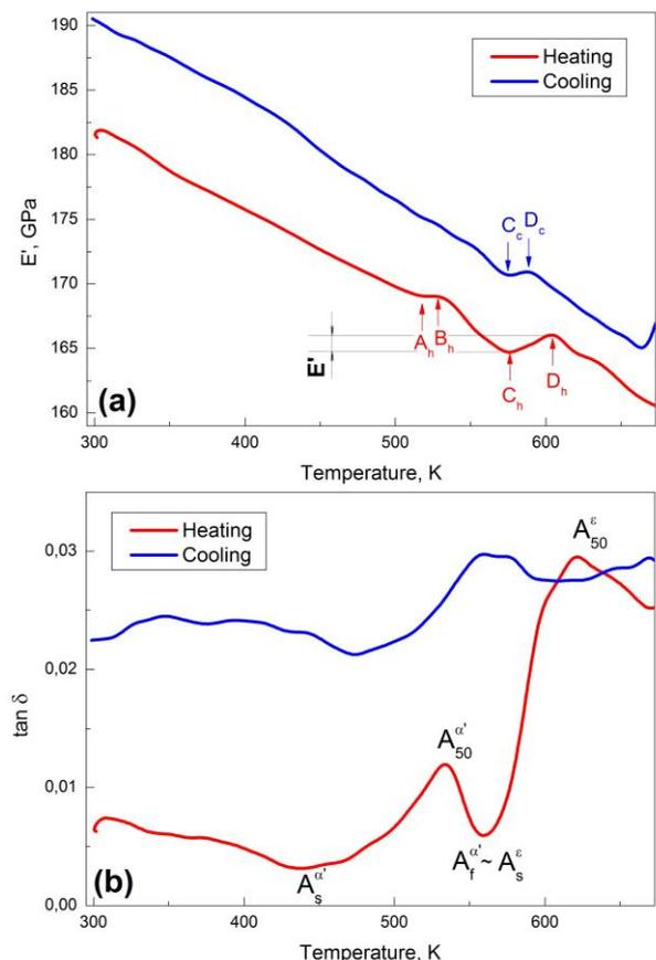
Fig. 2 DMA thermograms recorded in a heating-cooling cycle of 0\_MA\_700 specimen: (a) variation of storage modulus with temperature; (b) variation of internal friction with temperature
