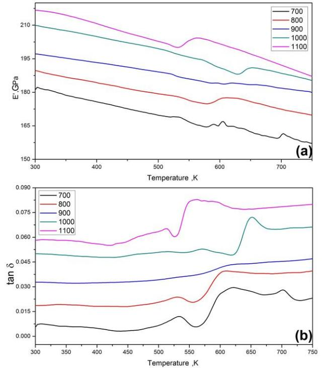
Fig. 3 Cumulative DMA thermograms illustrating the effects of heat treatment temperature (given in the inset, in  $^{\circ}\text{C}$ ), on the behaviour of specimens 0\_MA, during heating: (a) variation of storage modulus with temperature; (b) variation of internal friction with temperature.
