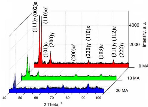
Fig. 10 Characteristic XRD patterns of the specimens heat treated at 1373 K
