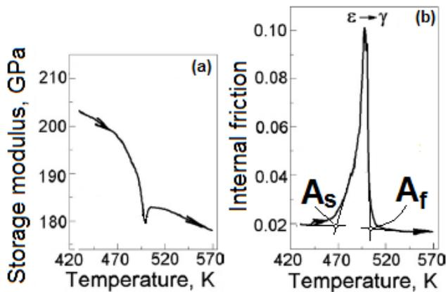
Fig.1 Typical schematic DMA thermogram recorded during the heating of a Fe-Mn alloy: (a) storage modulus variation with temperature; (b) internal friction variation with temperature.
