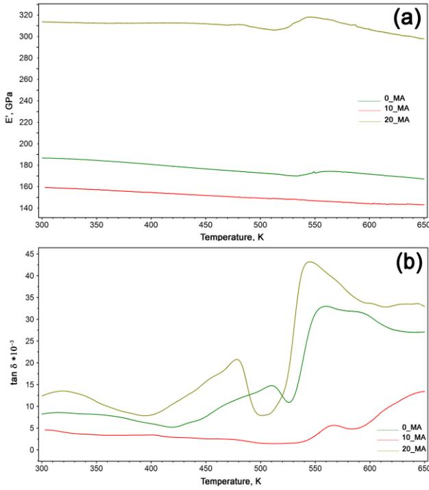
Fig. 4 DMA thermograms recorded on the specimens which were solution treated at 1373 K, illustrating the effects of MA fraction: (a) variation of storage modulus with temperature; (b) variation of internal friction with temperature
