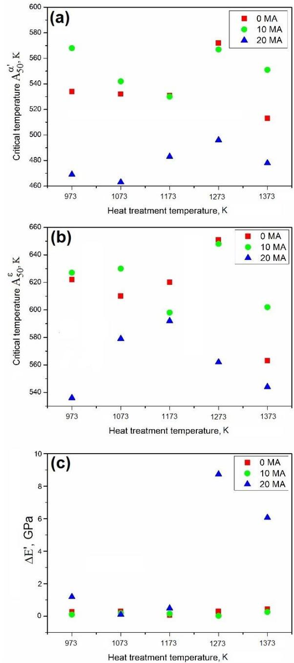
Fig. 5 Summary of the effects of solution treatment temperatures and MA fraction on the variation of characteristic parameters of DMA thermograms: (a)  $A_{50}^{\alpha'}$ ; (b)  $A_{50}^\varepsilon$  and (c)  $\Delta E'$
