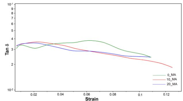
Fig. 9 Isothermal variations of average values of internal friction of the specimens heat treated at 937 K and tested at the temperature  $T_2$ , illustrating the effects of MA fraction.
