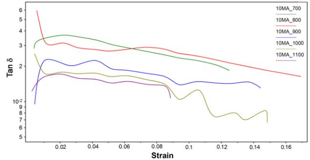
Fig. 8 Isothermal variations, at temperature  $T_2$  ( $A_s^E < T_2 < A_{50}^E$ ), of the average values of internal friction ( $\tan \delta$ ) of specimen 10\_MA
