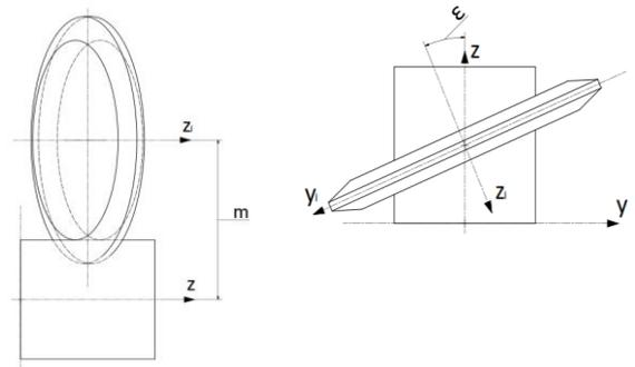
Fig. 4. Positioning parameters between tool and worm blank
