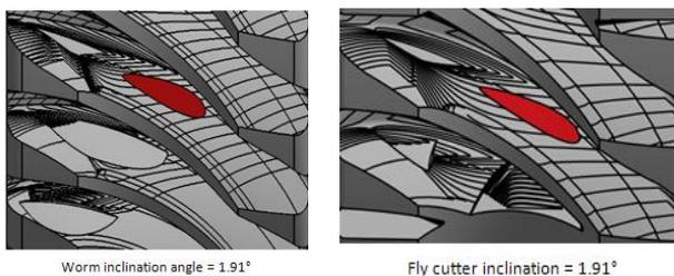
Fig. 12. Contact pattern modification due to worm inclination angle
