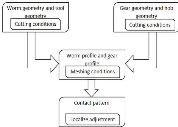
Fig. 2. Algorithm for contact pattern simulation, [3]
