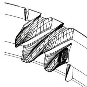
Fig. 9. Resulting worm gear tooth
