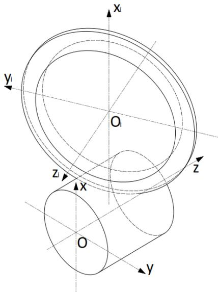
Fig. 3. Tool and worm blank and their coordinate systems
