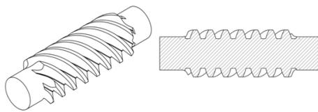
Fig. 6. ZK worm generated with profile resulted from presented methodology
