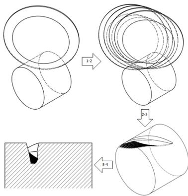
Fig. 5. Steps of grinding process simulation using CAD software
