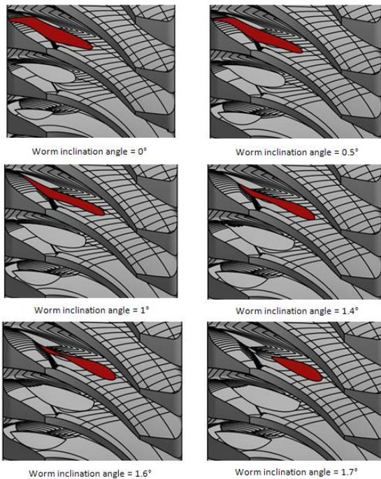
Fig. 11. Contact pattern modification due to worm inclination angle
