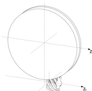
Fig. 8. Worm gear and fly cutter positioning
