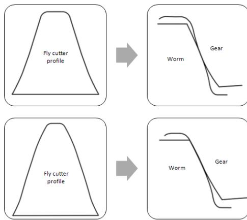
Fig. 10. Fly cutter profile influence on contact pattern
