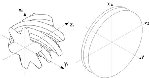
Fig. 7. Fly cutter and worm gear blank bodies
