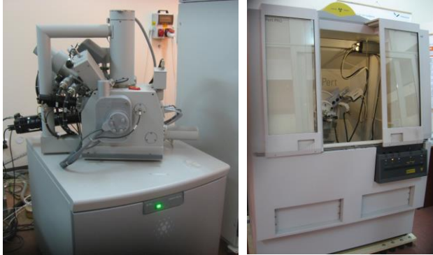
Fig. 2. Structural analysis equipments: a) SEM QUANTA 200 3D DUAL BEAM b) X'Pert Pro MPD Diffractometer
