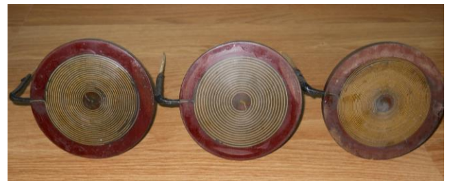
Fig.2. Shape of induction coils used in the experimental research: a) induction coil without concentrator; b) induction coil with field concentrator; 1-support plate; 2 - active plate; 3 - workpiece ; 4 - inductor; 5 - insulated plate; C - field concentrator.
