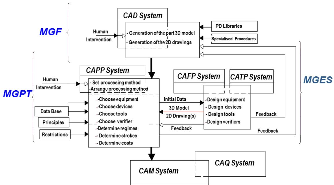
Fig. 1. The Modules of a standard generative CAPP system
