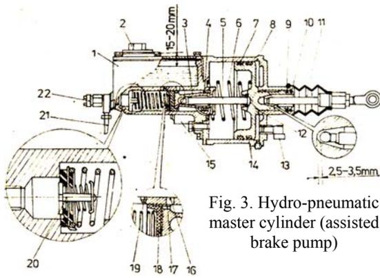
Fig. 3. Hydro-pneumatic master cylinder (assisted brake pump)
