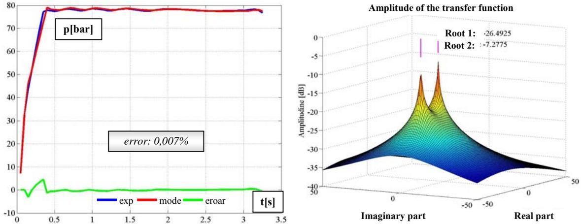
Fig. 7. Characteristic features of the mathematical model, and the time history of the brake cylinder's pressure as a function of the distributor's input pressure (global model) - ARX algorithm
