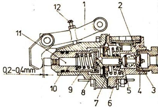
Fig. 4. Compressed air distributor
