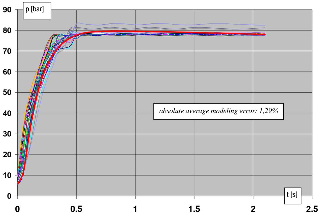
Fig. 8. Generalized, global model of the time history of the brake cylinder's pressure as a function of the distributor's input pressure
