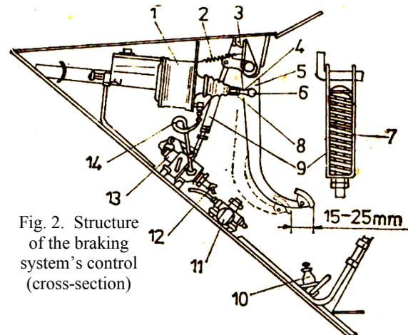
Fig. 2. Structure of the braking system's control (cross-section)
