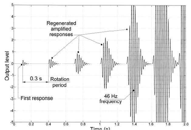
Fig.2. Dynamic response with +0.001 gain in the feedback loop 2 (negative synthetic damping)
