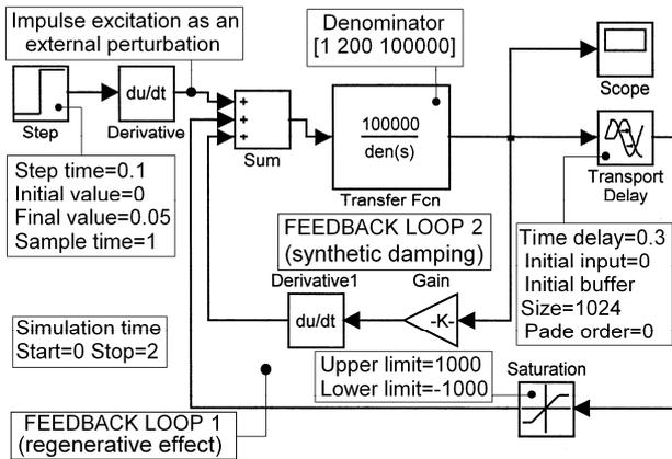
Fig.1. A Matlab/Simulink model of chatter based on regenerative effect. Chatter correction using negative feedback in feedback loop 2
