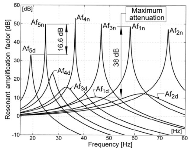
Fig. 9. The PDA efficiency in frequency domain, mirrored in the evolution of the resonant amplification factor (the magnitude in decibels)
