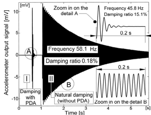
Fig. 7. The PDA efficiency (optimal tuning) in time domain, mirrored in viscously damped free response (I). Viscously damped free response of the cantilever beam without PDA (II).
