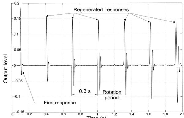
Fig.3. Dynamic response with  $-0.001$  gain in the feedback loop 2 (active positive damping)
