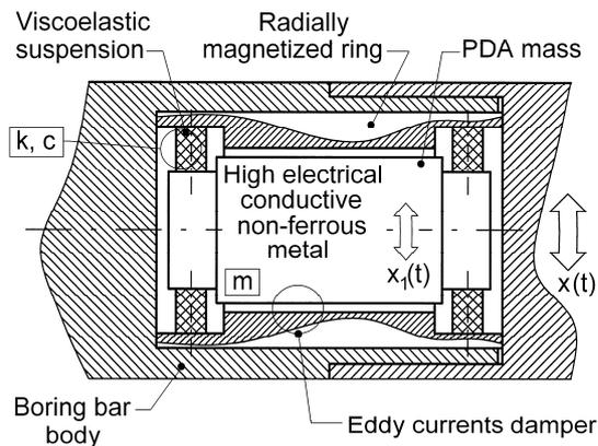
Fig. 10. The PDA setup inside the boring bar
