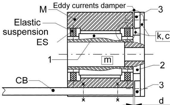
Fig. 5. Cantilever beam setup with passive dynamic absorber
