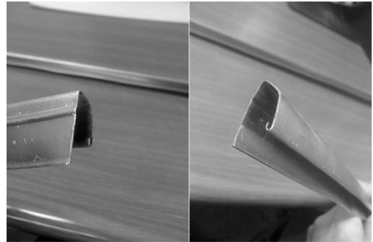
Fig. 18. The cross section of the aluminum car doorbelt in the confirmation experiment
