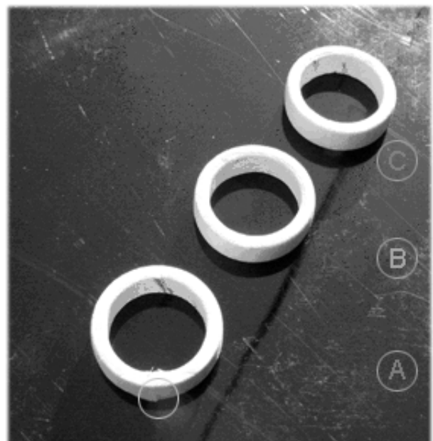
Fig. 2. The use of sodium silicate as a replacement of the infiltrant Z-bond 101
