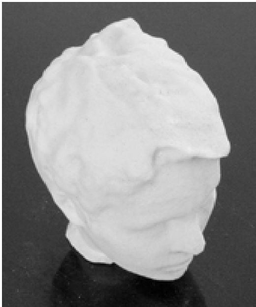
Fig. 3. Object made by the use of 3D printer Zprinter 310 Plus, from ZP131 powder, where the hardener layer of sodium silicate, solution 50%, was applied by brush
