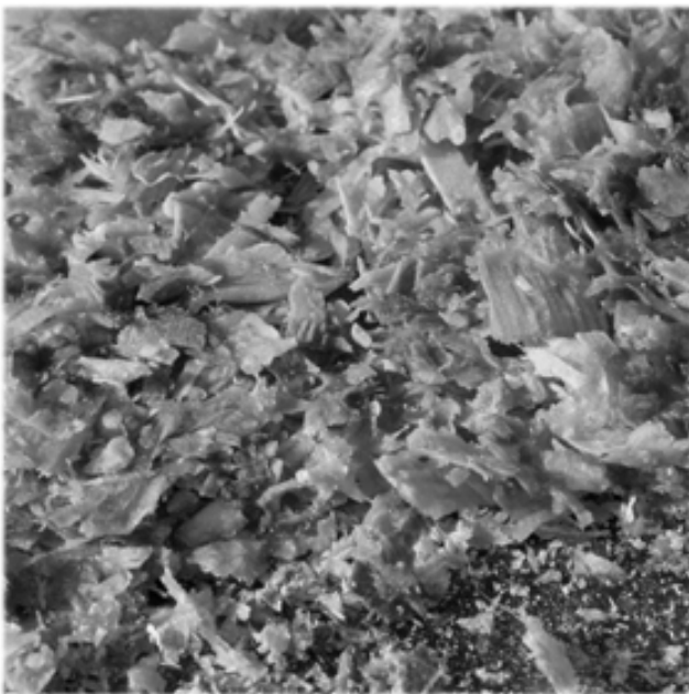
Fig. 7. Mixture of sawdust and water glass
