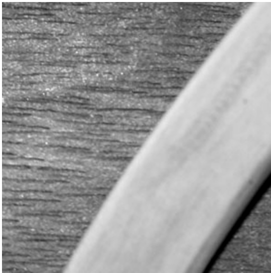
Fig. 12 – Crystals of sodium silicate revealed on veneer surface, which was treated with sodium silicate, after 5 months (in detail fig. 11)
