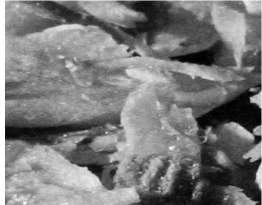
Fig. 8. Detailed mixture of sawdust and water glass where silicate granules can be observed
