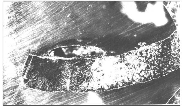
Fig. 2. OLT 35 after the action of the acid solution(B)
