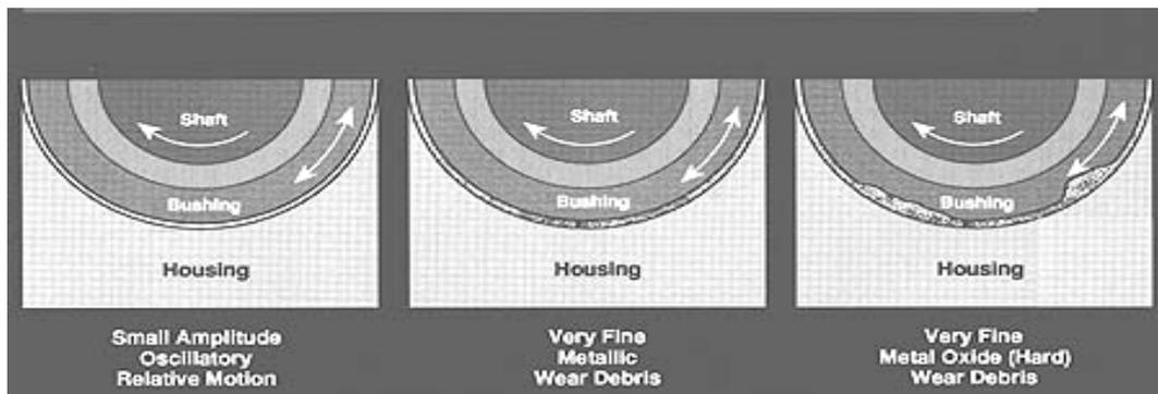
Fig. 10. The mechanism of fretting corrosion
