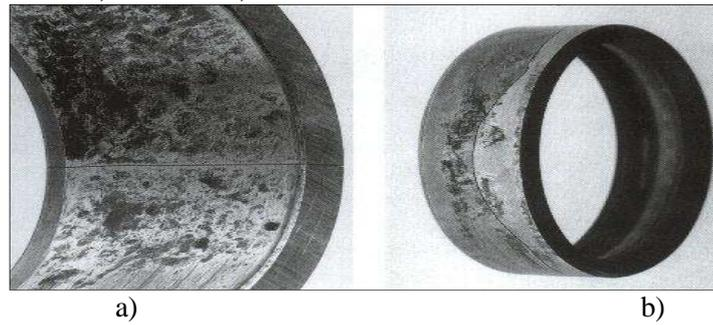
Fig. 9. a) The fretting corrosion has caused the cracking of spherical roller bearing inner ring; b) fretting corrosion has caused longitudinal crack in a deep groove ball bearing outer ring.
