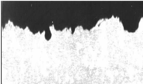
Fig. 3. OLT 35 after acid solution less inhibitors (A)
