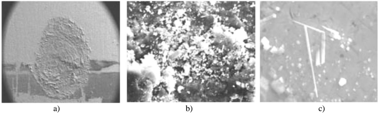
Fig. 6. a) Fretting scar; b) Wear particles formed in laboratory air; c) Wear particles under argon atmosphere
