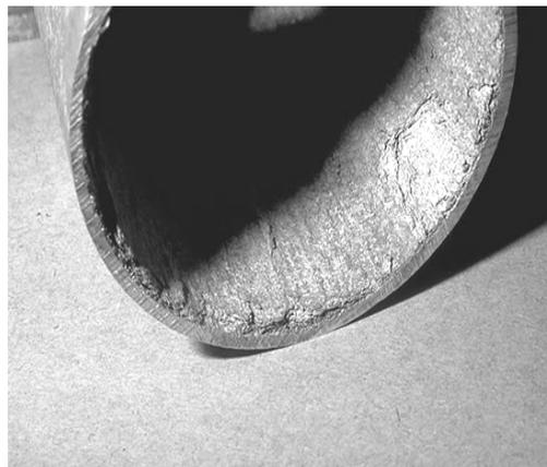
Fig. 7. Exfoliation corrosion morphology inside of formation of grooves, holes etc
