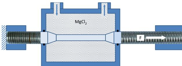
Fig. 1. Scheme of the SSRT testing, [own elaboration]
