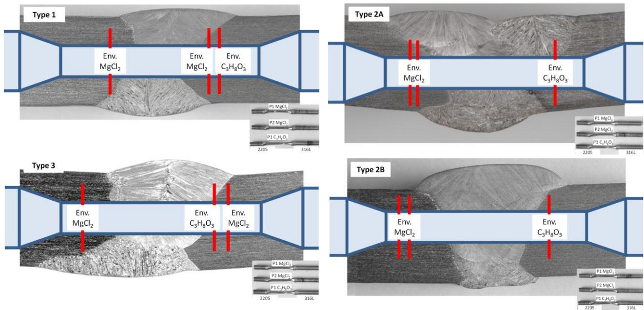
Fig. 4. Specimens fracture locations for different joint type, [own elaboration]
