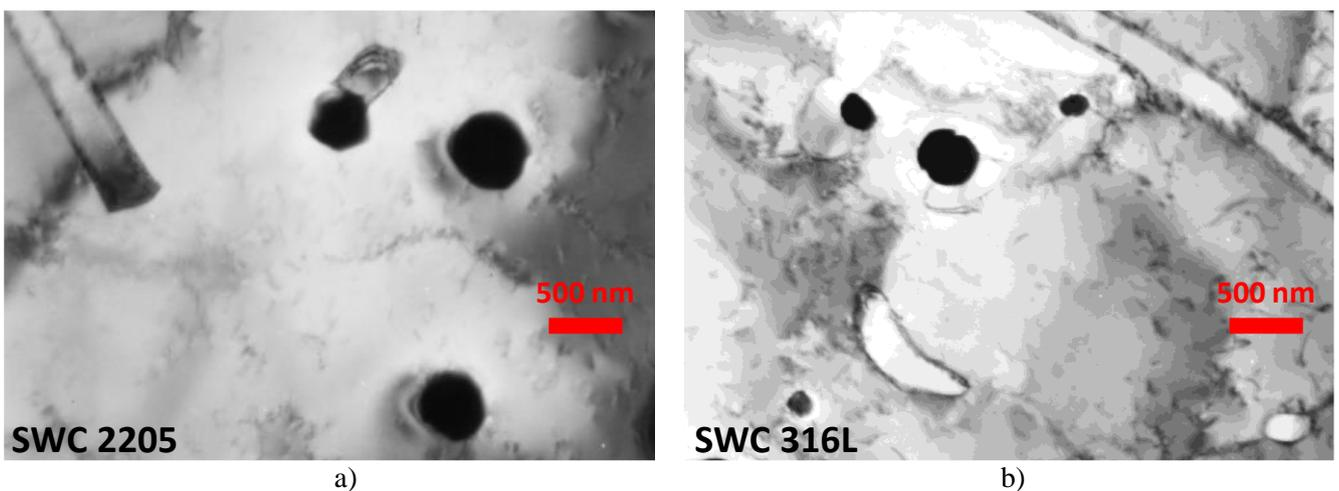
Fig. 7. M<sub>23</sub>C<sub>6</sub> carbide particles on the side: a) HAZ 2205, b) HAZ 316L of the type 3 joint, [own elaboration]
