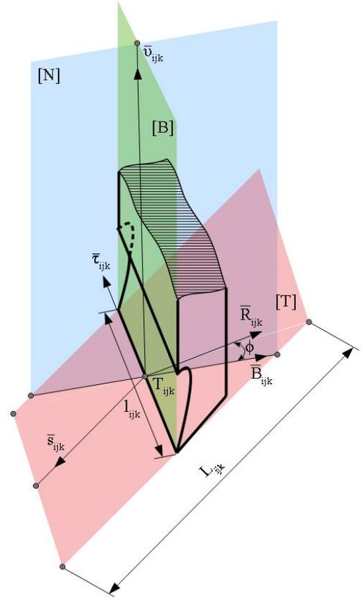
Fig. 3. The elementary fragment of tool tooth
