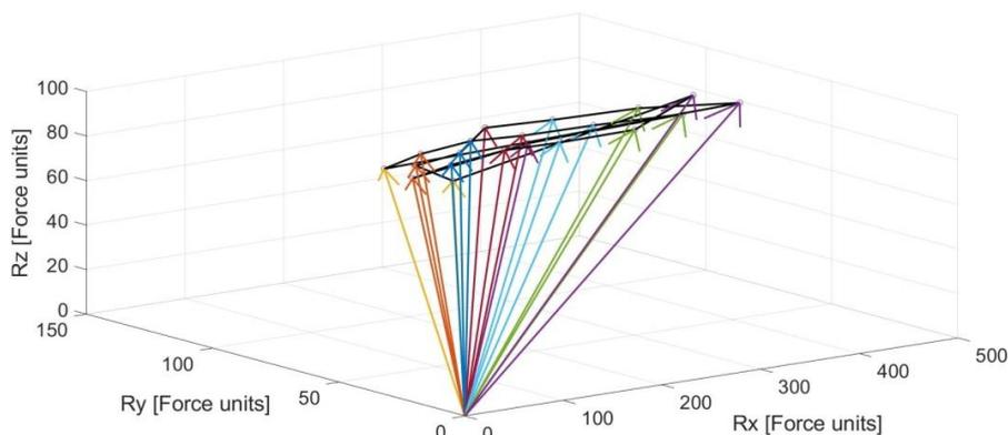
Fig. 6. Cumulated cutting force hodograph
