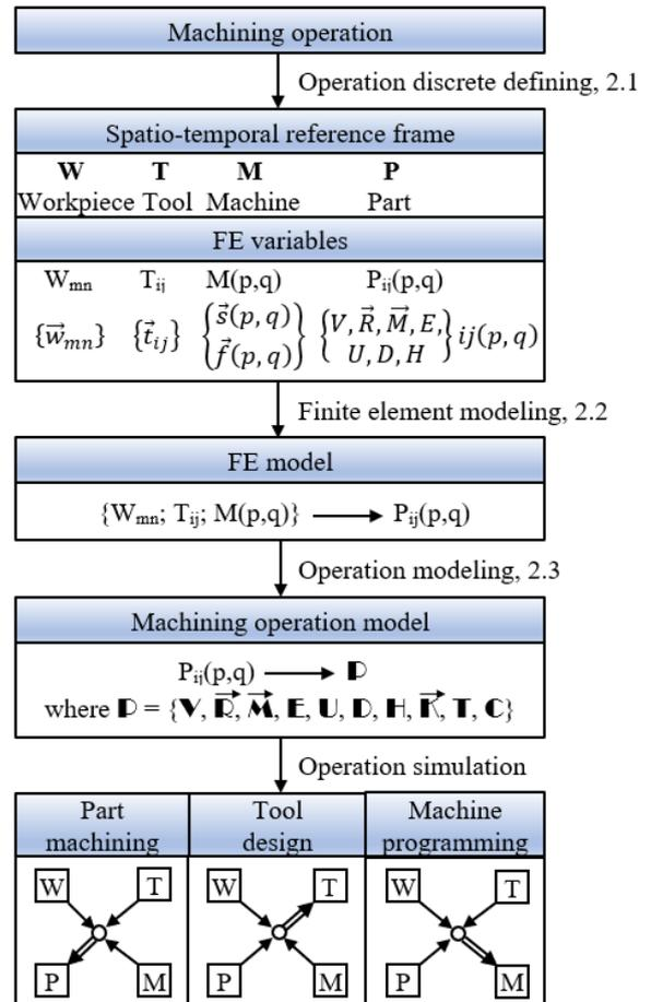
Fig. 8. Extending the model to other machining operations
