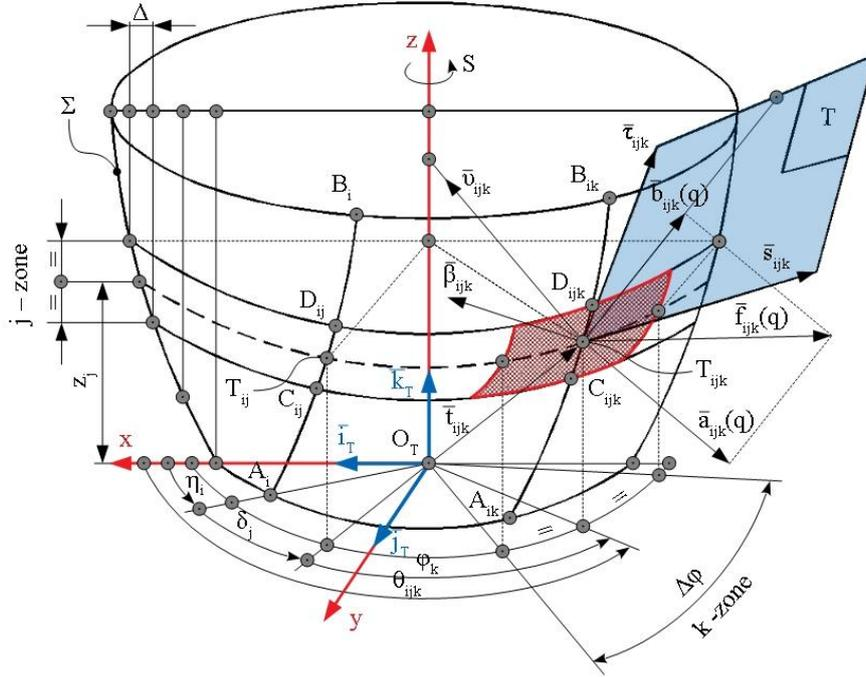
Fig. 1. Tool discrete definition
