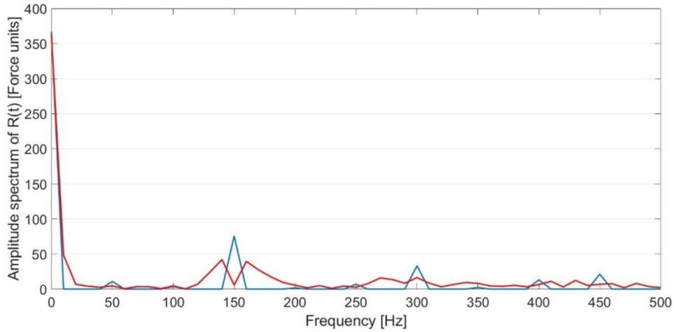
Fig. 7. Amplitude spectrum of cutting force R: tool with equidistant teeth (blue) vs. tool with successive teeth placed at different angular intervals (red)
