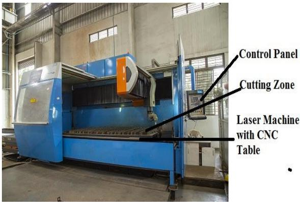
Fig. 1. Laser beam machine setup
