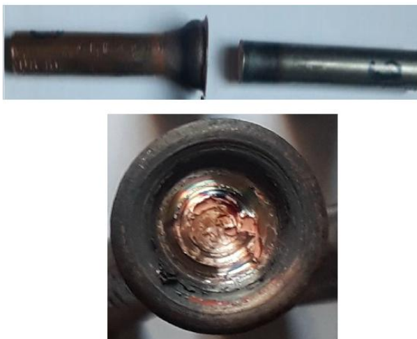
Fig. 8. Macrographic view of welded specimen, fractured by tensile test. Magnification of the trasversal section
