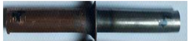
Fig. 2. Friction welded piece
