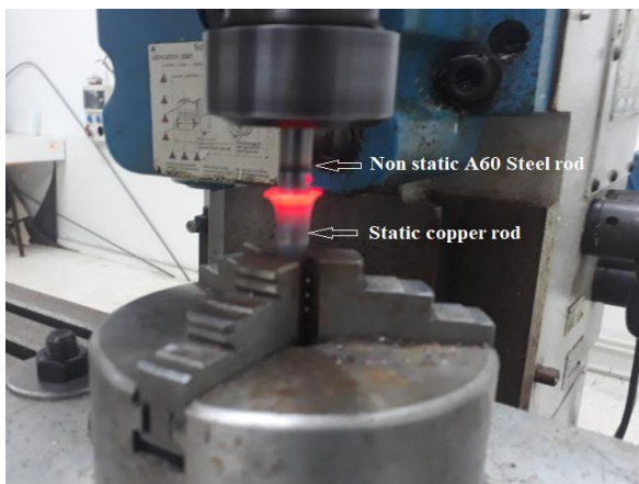
Fig.1. Friction welding of copper bar to A60 steel bar
