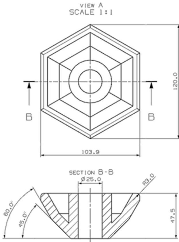
Fig. 5. Basic dimensions of Model 2
