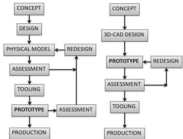
Fig. 1. On the left – traditional approach; on the right – construction using RP techniques, [5]
