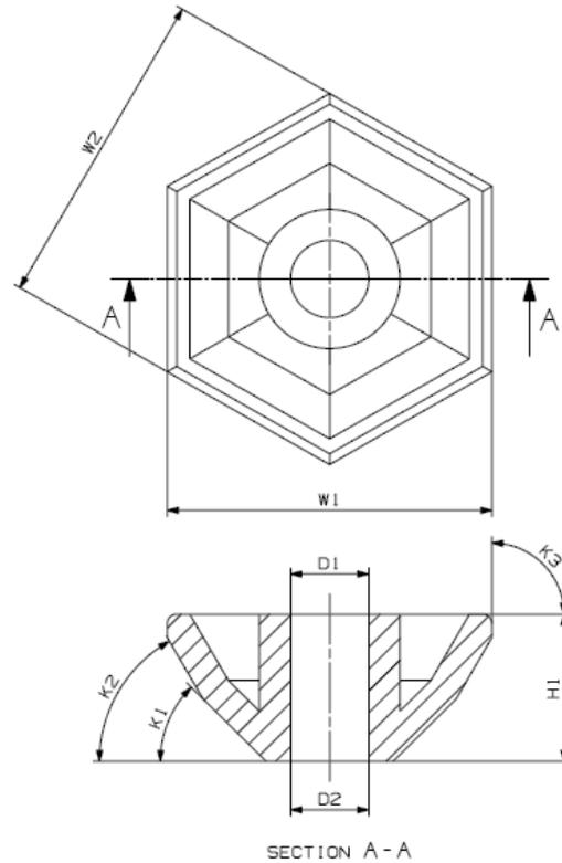
Fig. 10. Marking of dimensions measured in Model 2
