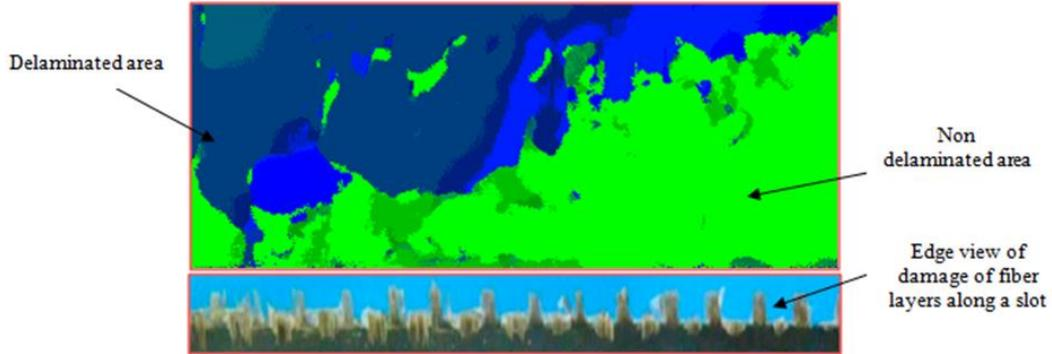
Fig. 4. Ultrasonic C-scan sample image of machined GFRP workpiece along a slot
