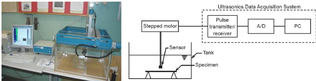
Fig. 3. Ultrasonic C-scan setup for measuring delamination damage
