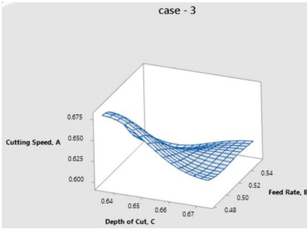
Fig. 7. Surface response plot for evaluation of optimal setting (case 3)
