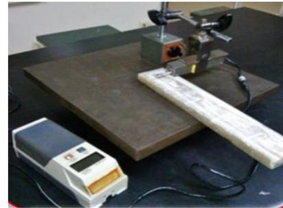
Fig. 2. Surface roughness measuring setup
