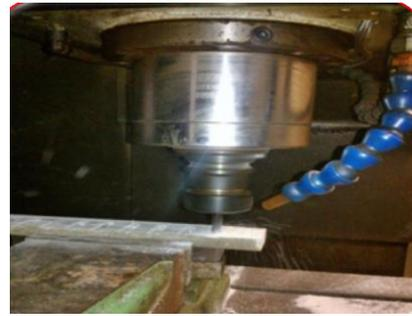
Fig. 1. GFRP work piece setting on CNC milling machine
