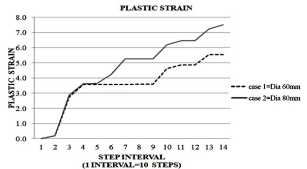
Fig. 5. Comparisons of strain rate distribution for case 1 and case 2
