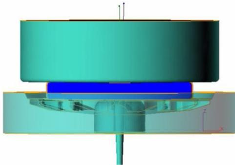
Fig. 2. Complete setup of the dies with work piece
