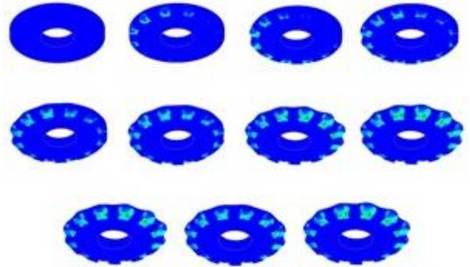
Fig. 4. The distribution of effective strain (PEEQ)
