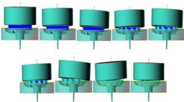
Fig. 3. Steps showing the development of gear in cold orbital forming
