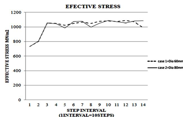
Fig. 8. Comparison of effective stress distribution for case 1 and case 2
