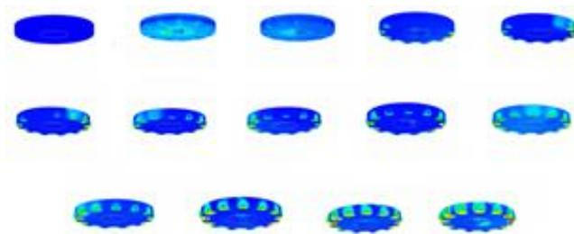
Fig.7. Equivalent Stress distribution of the deforming billet with time
