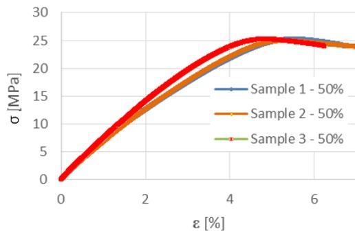
Fig. 4. Tensile strength of PLA printed sample – 50% infill rate
