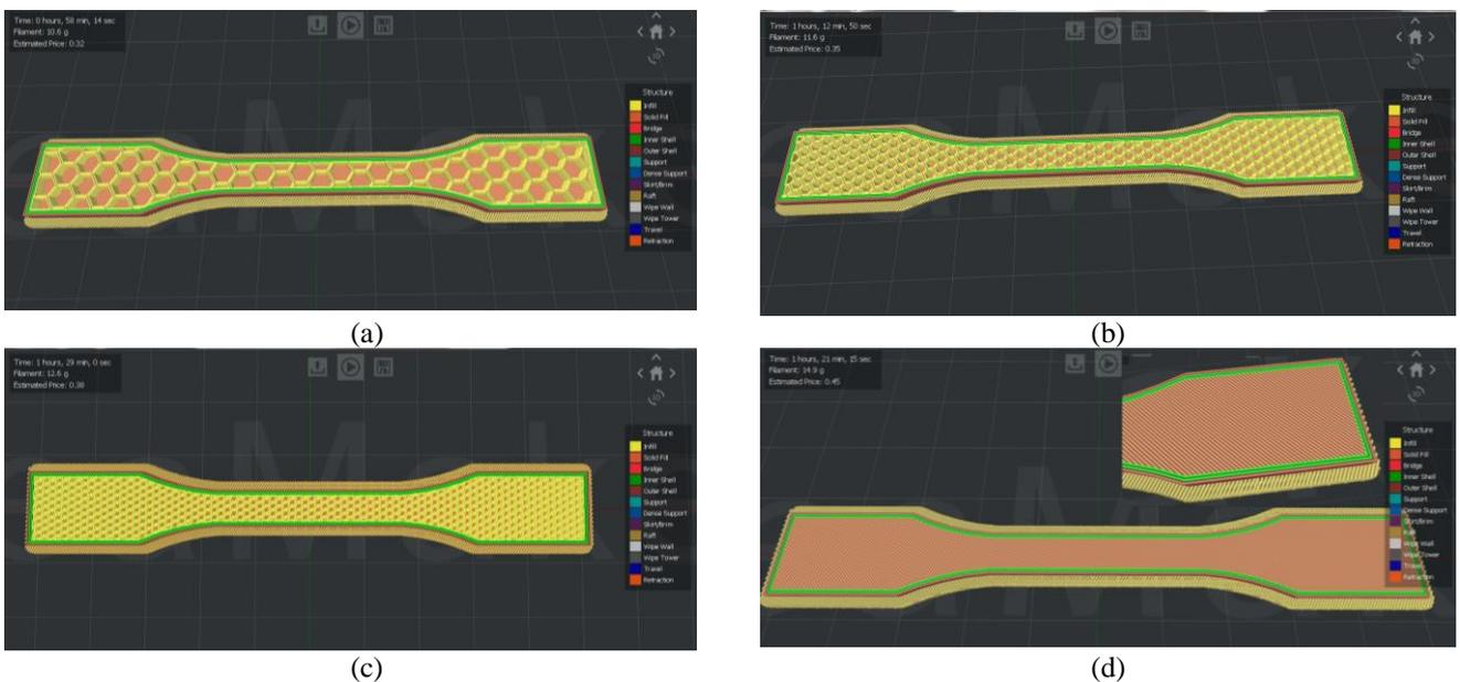
Fig. 2. Infill of PLA sample, Honeycomb type: (a) 25% (b) 50%; (c) 75%; (d) 100%
