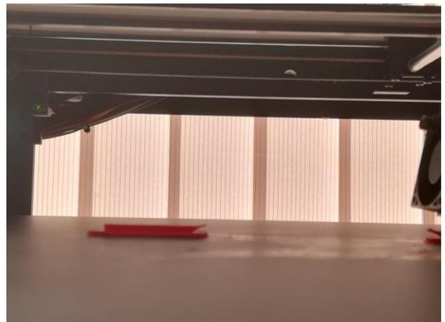
Fig. 13. Deformation by thermal shrinkage of the sample pick
