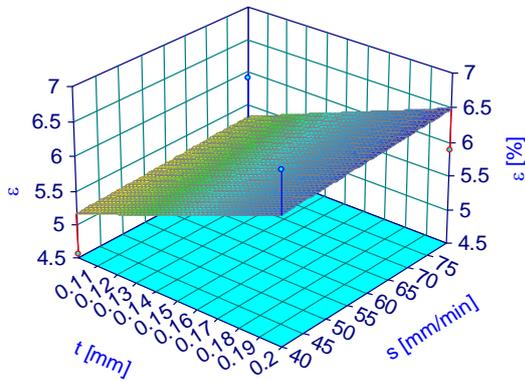
Fig. 10. The regression equation for PLA samples elongation printed on-edge
