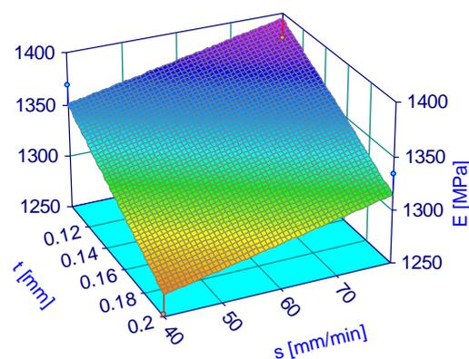
Fig. 9. The regression equation for PLA samples elasticity modulus printed on-edge
