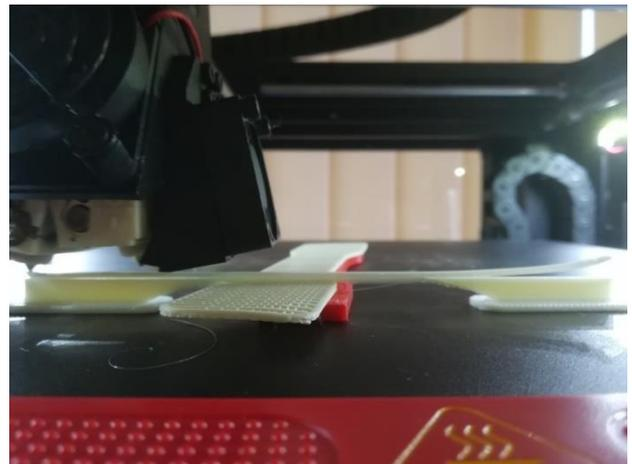
Fig. 12. Deposited layers' delamination through 3D printing
