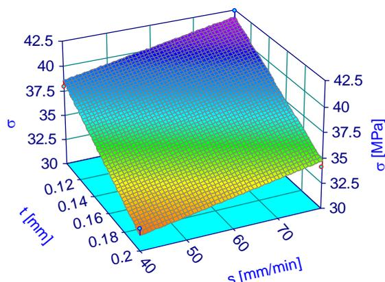
Fig. 8. The regression equation for PLA samples tensile strength printed on-edge
