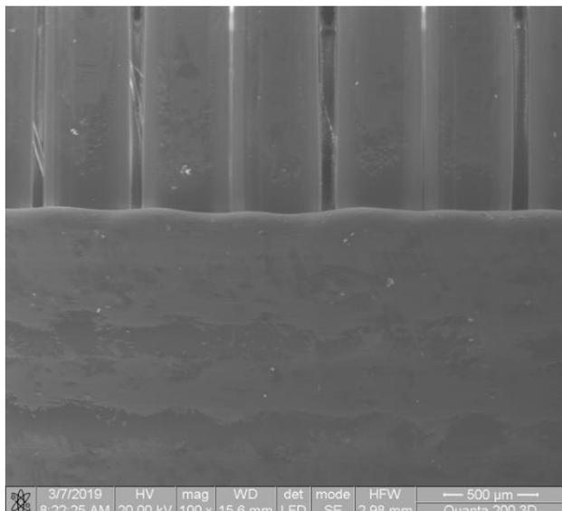
Fig. 7. SEM image of 3D printed PLA, „honeycomb” type
