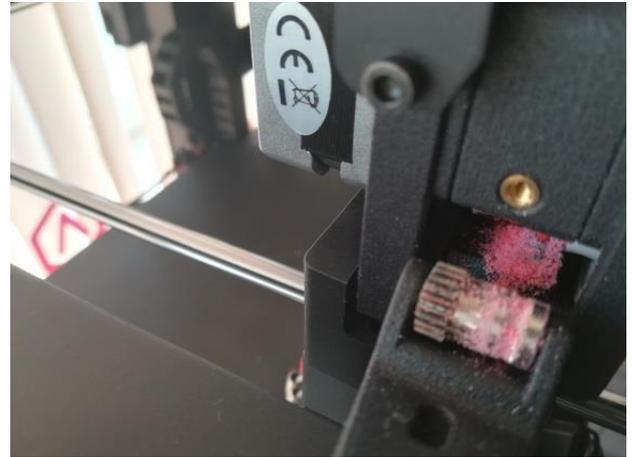
Fig. 11. Drive area clogging of the wire with the material chips
