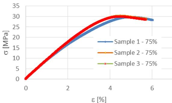
Fig. 5. Tensile strength of PLA printed sample – 75% infill rate
