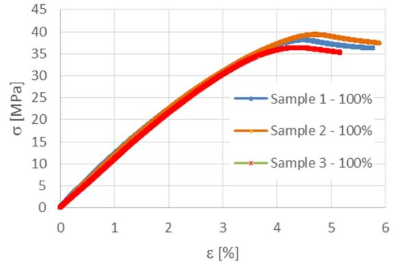
Fig. 6. Tensile strength of PLA printed sample – 100% infill rate
