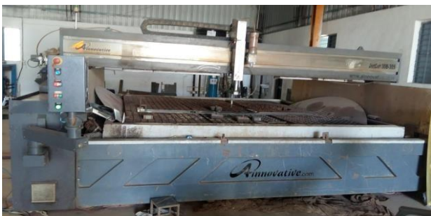
Fig. 3. AJM Setup (Courtesy: M/s Shree jiAinnovative International Ltd.)
