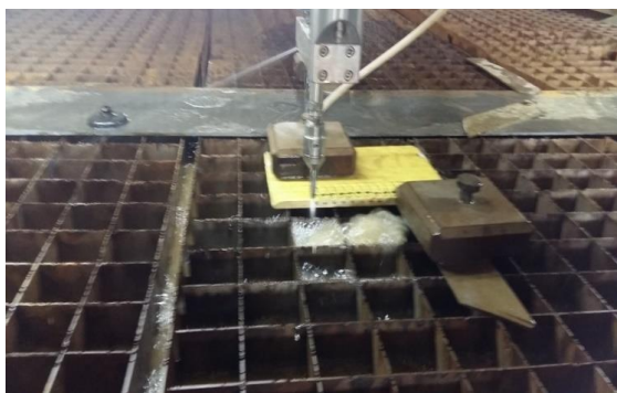
Fig. 4. Machining of Kevlar 49 epoxy composite by AWJM
