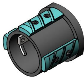
Fig. 4. Assembled view of a combined tool for expanding holes with inclination of the cutting edge 60^\circ
