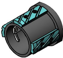
Fig. 3. Assembled view of a combined tool for expanding holes with inclination of the cutting edge 30^\circ
