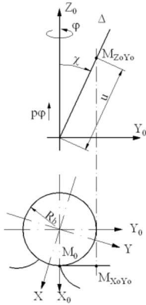
Fig. 9. Reference systems and crossing section of the involute worm
