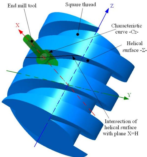
Fig. 7b. Tool's working position
