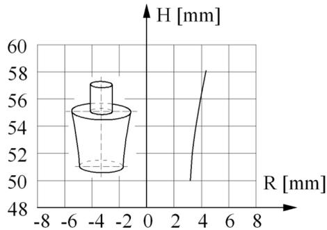
Fig. 10. Axial section of end mill tool
