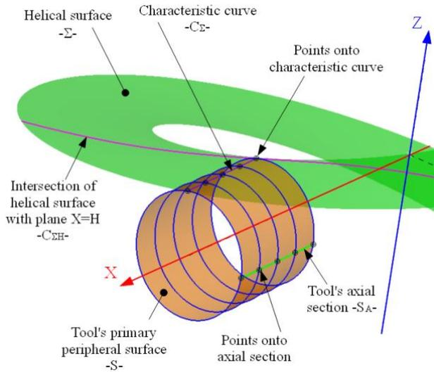
Fig. 6. Tool's primary peripheral surface; characteristic curve; axial section
