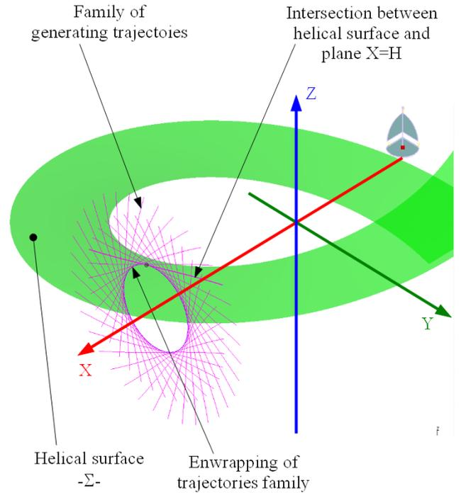
Fig. 5. Intersection between helical surface and planes; family of  $C_{\Sigma}$  curves; enwrapping of family
