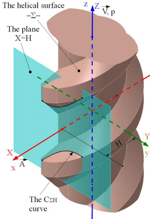
Fig. 2. Helical surface; the plane  $X=H$ ; the reference systems
