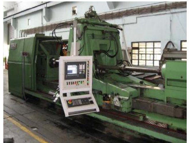
Fig. 2. The flow-forming machine (Make: Leifeld, Germany; Model: ST 56-75 CNC)
