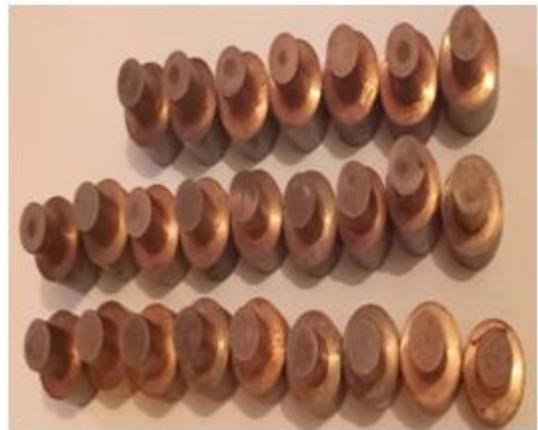
Fig. 3. Tool electrodes used for experiments
