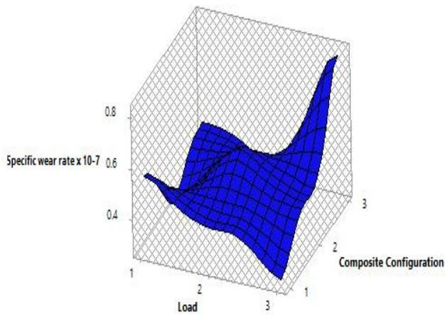
b) specific wear rate vs composite configuration, load
