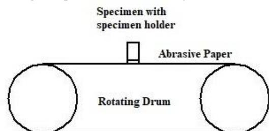
Fig. 3. The schematic arrangement of two body abrasion
