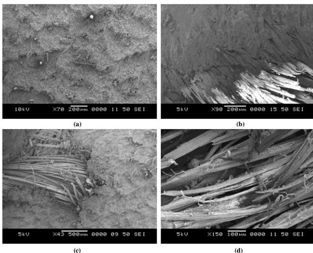
Fig. 9. Surface morphology showing wear mechanisms of constituents of the composite
