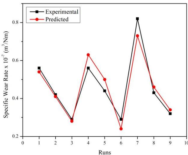
Fig. 7. Comparison of experimental and predicted specific wear rate
