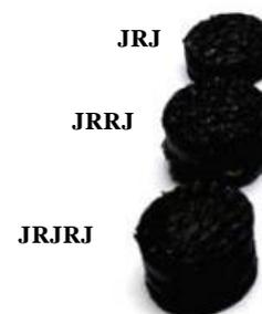
Fig. 2. Specimens for two body abrasion test
