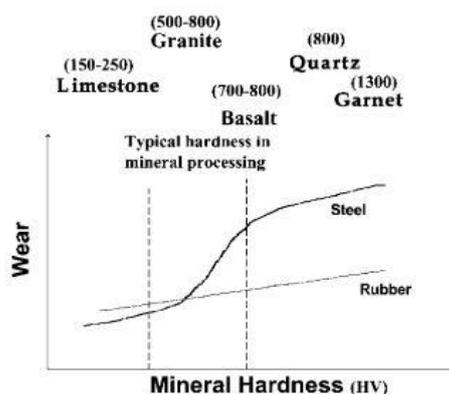
Fig. 1. Variation of wear rate for steel and rubber for different erodents (Sare, Mardel and Hill, 2001)
