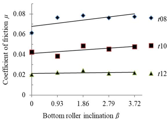
Fig. 10. CF at top roller versus  $\beta$  ( $\alpha=0^\circ$ )
