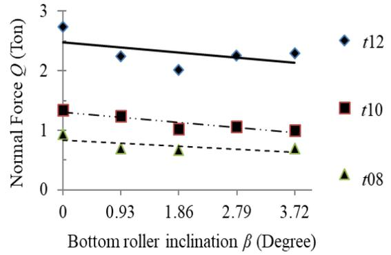
Fig. 8b. Total normal force ( $Q$ ) for different bottom roller inclination  $\beta$  and thickness  $t$  ( $\alpha=0^\circ$ )
