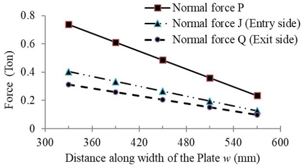
Fig. 7. Normal Forces along the width of plate at each roller-plate interface ( $t=10$ ,  $\beta=1.86^\circ$ ,  $\alpha=0^\circ$ )
