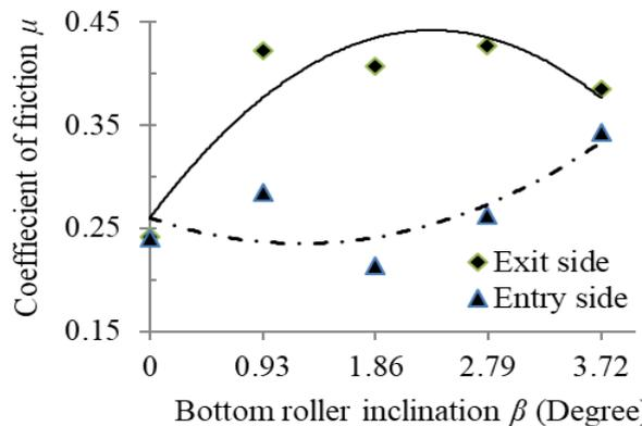
Fig. 9b. CF on entry and exit side versus  $\beta$  ( $t=10$ mm,  $\alpha=0^\circ$ )
