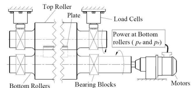
Fig. 2c. Measurement of force and power during bending (Kagzi and Raval, 2018)
