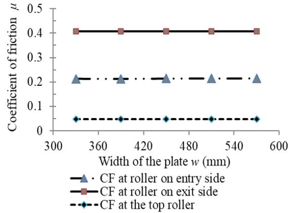
Fig. 8.c. CF obtained along the plate width for ( $t=10$ mm,  $\beta=1.86^\circ$ ,  $\alpha=0^\circ$ )
