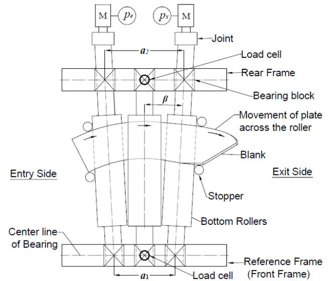
Fig. 2b. Movement of plate and experimental setup for conical bending
