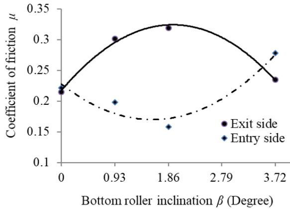
Fig. 9c. CF on entry and exit side versus  $\beta$  ( $t=8\text{mm}$ ,  $\alpha=0^\circ$ )
