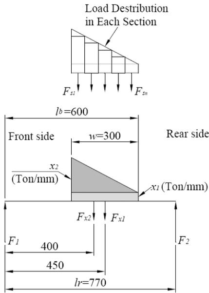
Fig. 4b. Assumed force distribution on the top roller (All dimension are in mm)
