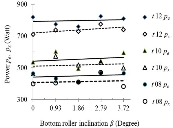
Fig. 6. The power measured during continuous bending process
