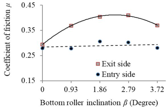
Fig. 9a. CF on entry and exit side versus  $\beta$  ( $t=12$ mm,  $\alpha=0^\circ$ )
