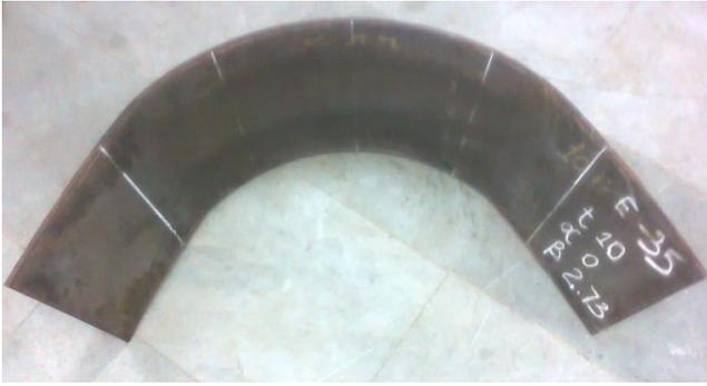
Fig. 3b. Plate after conical bending for one of the case ( $t=10\text{mm}$ ,  $\beta=2.73^\circ$ )
