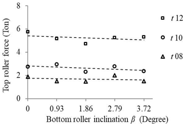
Fig. 5. The forces measured at the top roller during continuous bending process
