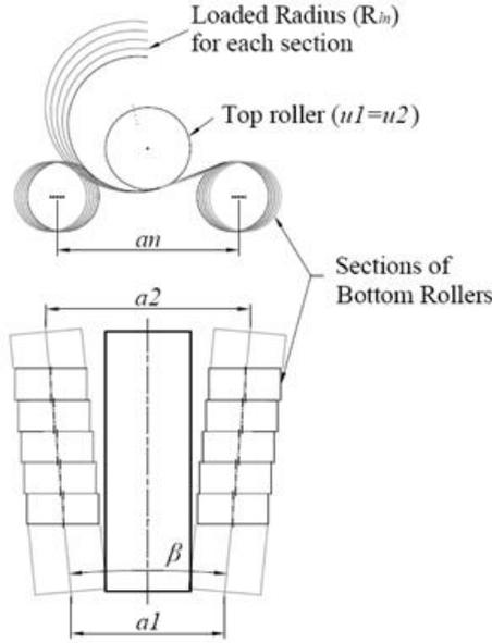
Fig. 4a. Bending along with assumed to be divided in different section
