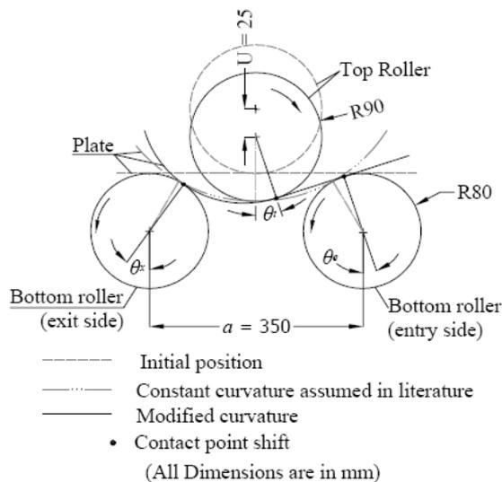
Fig. 1. Pyramid type three roller bending process (Kagzi and Raval, 2018)
