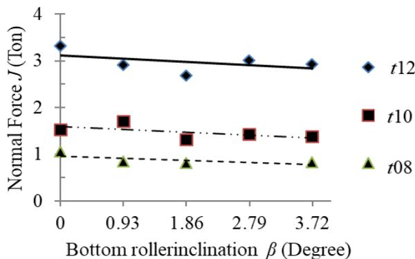
Fig. 8a. Total normal force ( $J$ ) for different bottom roller inclination  $\beta$  and thickness  $t$  ( $\alpha=0^\circ$ )
