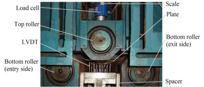
Fig. 2a. Experimental set up used for conical bending (Kagzi and Raval (2018))
