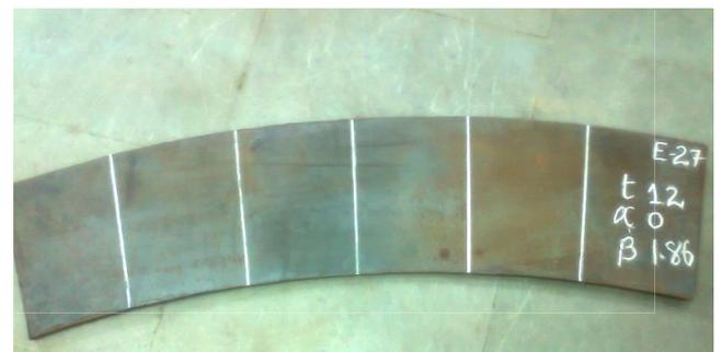
Fig. 3a. Initial plate for conical bending for one of the case ( $t=12\text{mm}$ ,  $\beta=1.86^\circ$ )
