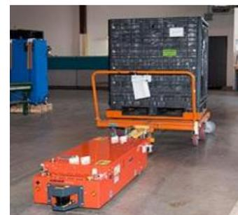
Fig. 2. Tow AGV with automatic hitch [19]
