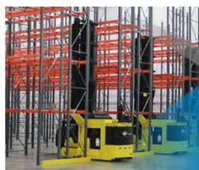
Fig. 9. High-bay racking AGV [8]
