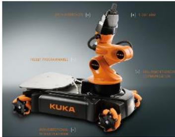
Fig. 5. Unit Load AGV with a Robotic Arm, [5]
