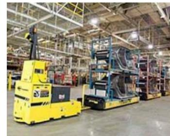
Fig. 1. Tow AGV with manual hitch [16]
