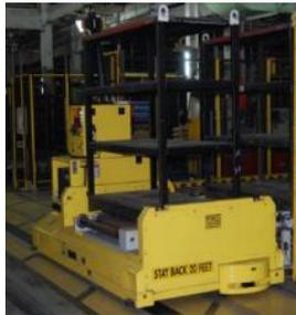
Fig. 3. Unit Load AGV with a Conveyor Deck [6]
