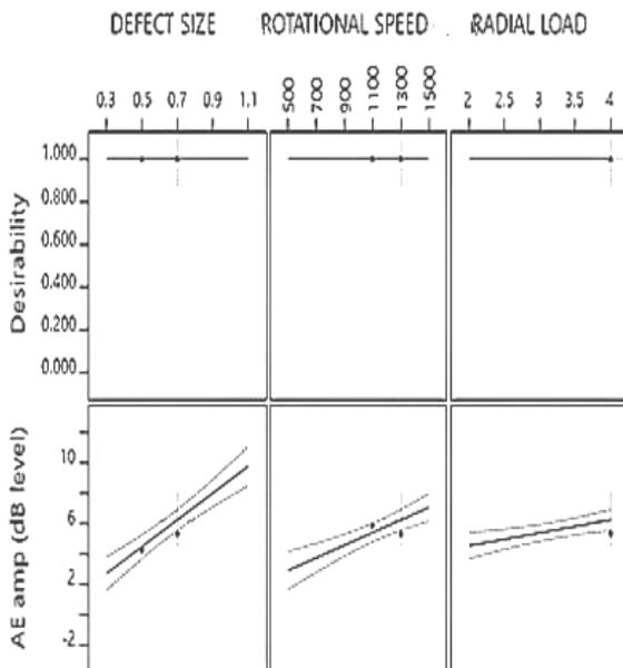
Fig.7. Optimization of AE amplitude
