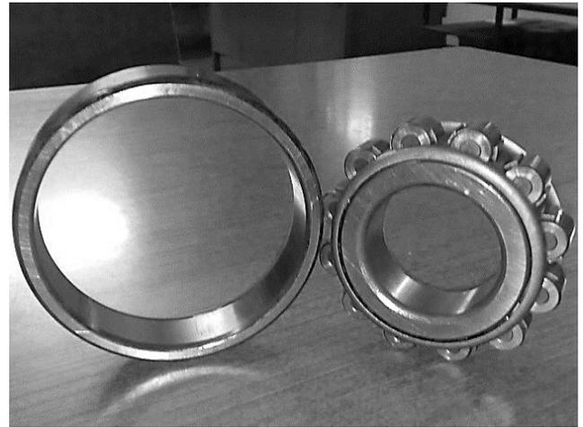
Fig .4. Test bearing
