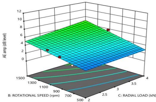
Fig. 6. (c). Effect of rotational speed and Radial load on AE amplitude
