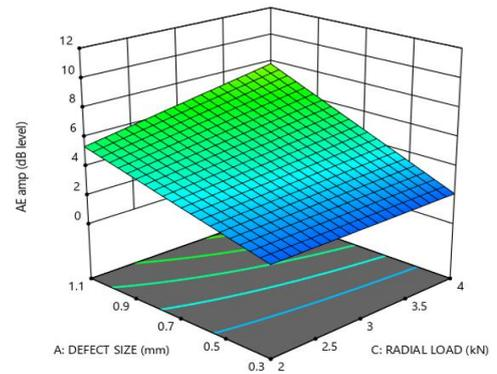
Fig. 6. (d). Effect of defect size and radial load on AE amplitude
