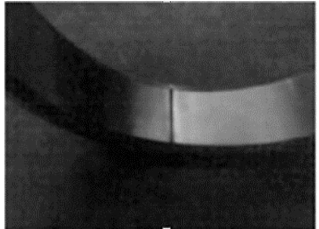
Fig. 3. Outer race seeded line defect
