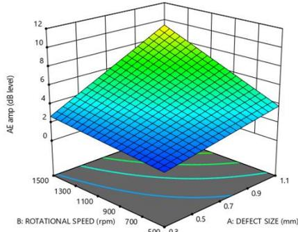
Fig. 6. (b). Effect of rotational speed and defect size on AE amplitude
