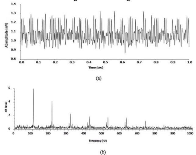
Fig. 5. AE (a) Time wave (b) Frequency spectrum of test conditions L2-D3-N6
