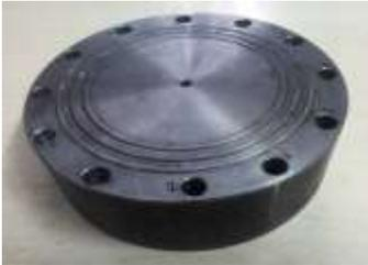
Fig. 3. Fabricated male die
