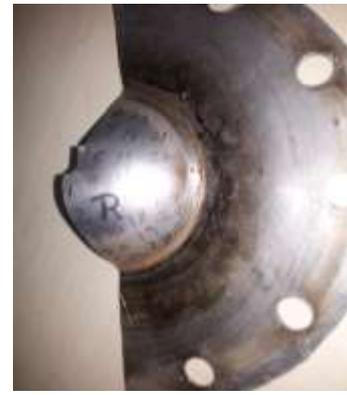
Fig. 20. Right Portion of Super plastically Formed Sheet Metal
