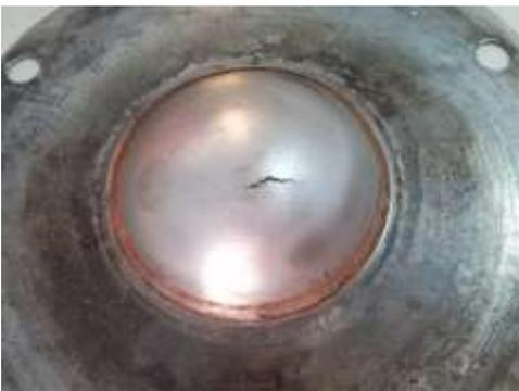
Fig. 16. Crack on Formed Aluminum Sheet Metal
