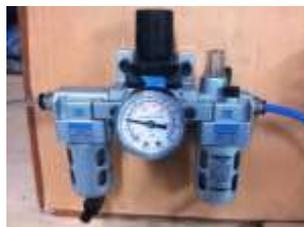
Fig. 13. Constant Pressure Gauge at 3.5bar
