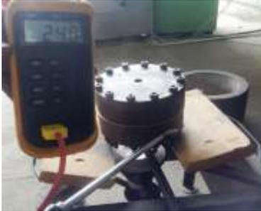
Fig. 11. Temperature Measuring with Pyrometer
