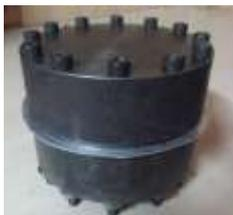
Fig. 7. Assembly of Dies with Sheet metal
