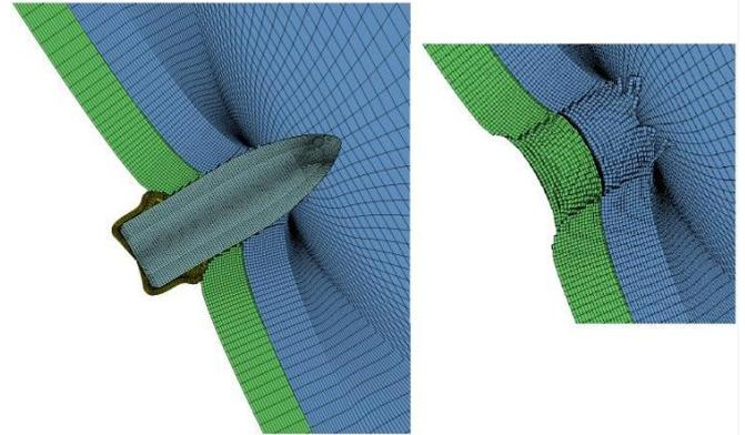
Fig. 8. Layered plate penetration – Final state of analysis
