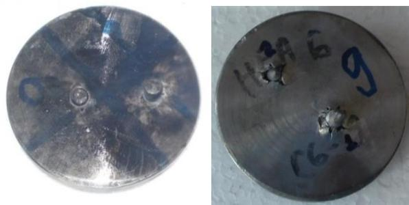
Fig. 2. HEA 6 sample, plate no. 9, thermal untreated (impact face, verso)
