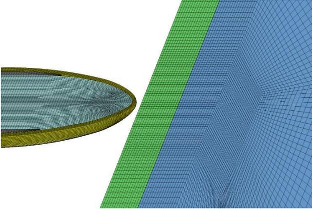
Fig. 7. Finite elements mesh – Impact area detail
