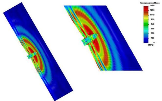
Fig. 9. Model von Misses stress – Final state of analysis
