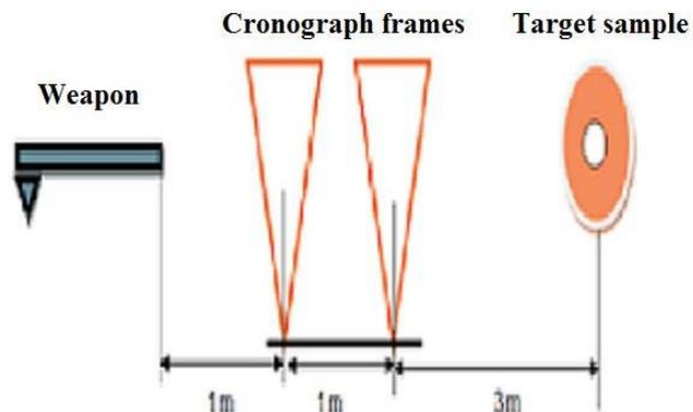
Fig. 1. Testing configuration
