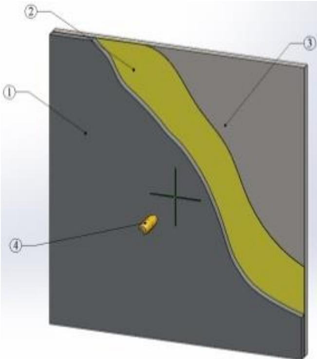
Fig. 5. Physic model of the HEA – Steel layered structure that suffers an impact with 7.62 mm armor piercing incendiary bullet
