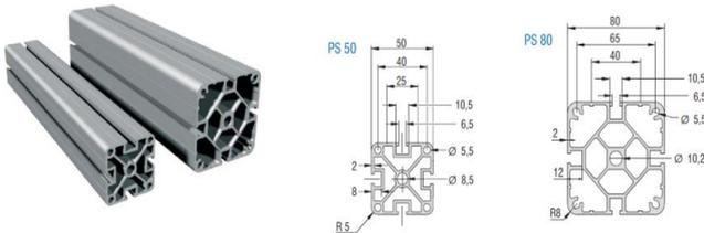
Fig. 5. Vertical profile supports [3]
