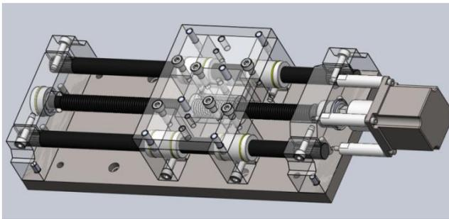
Fig. 10. Schematic of the driveline
