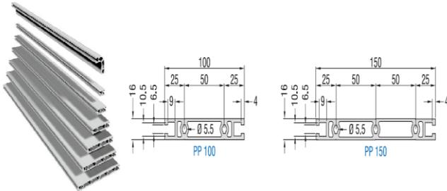
Fig. 6. Profile of lateral reinforcement [3]
