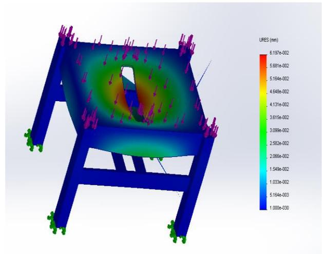
Fig. 8. The analysis of the deformations with a finite element analysis (FEA)
