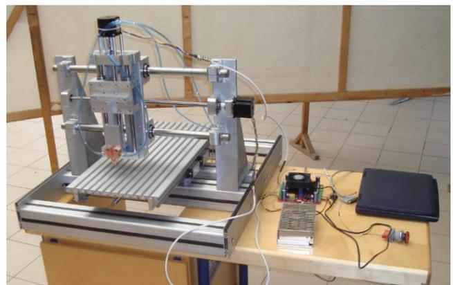
Fig. 2. Built model of the rapid freeze prototyping machine (version 1).
