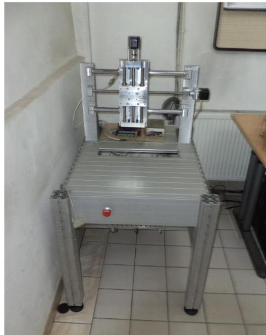
Fig. 4. Built model of the rapid freeze prototyping machine (version 2)
