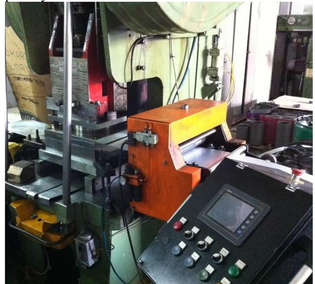
Fig. 7. A PLC controlled eccentric press used in the experiments
