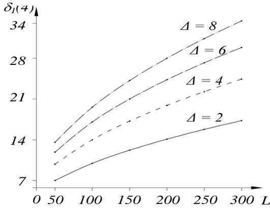
Fig. 7. Graph of dependences of  $\delta_l(4)$  on  $L$  under different values of  $\Delta$  for a scheme, given in Fig. 5
