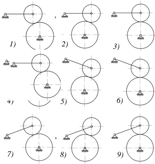
Fig. 2. Schemes of reciprocal location of working shafts before the beginning of technological process, when working shafts are in reciprocal contact
