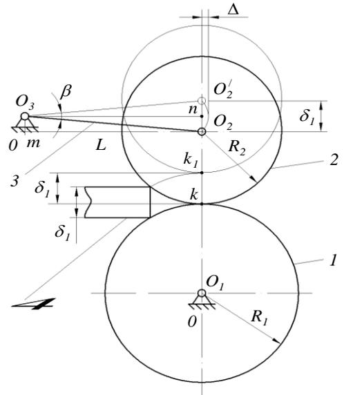
Fig. 5. Design scheme of rolling pair to determine the location and the length of a lever for the second approach to solution of the problem
