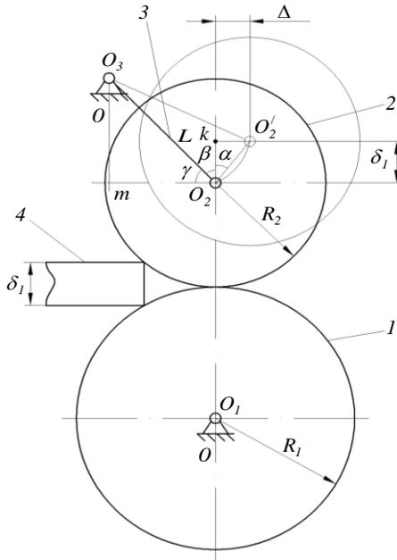
Fig. 10. Design scheme to determine the coordinates of the point of fixation of a lever on base box
