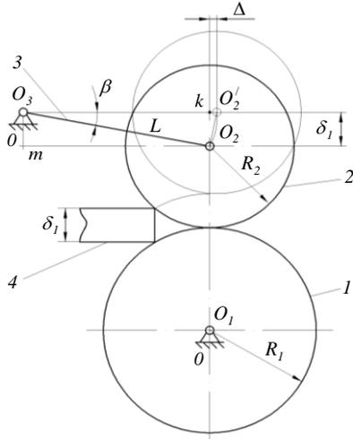
Fig. 4. Design scheme of rolling pair to determine the location and the length of a lever for the first approach to solution of the problem
