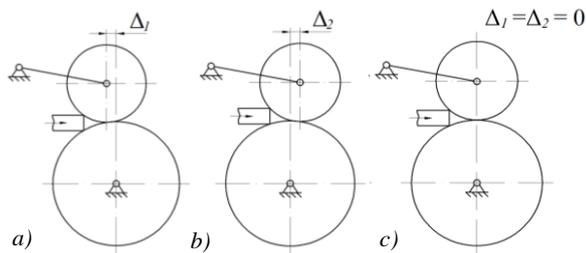
Fig. 3. Types of initial displacements in rolling pairs: a) displacements in direction of feeding of processed material; b) displacements in opposite direction of feeding of processed material; c) the case without displacement
