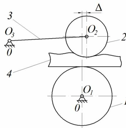
Fig. 1. Scheme of rolling pair with the center of movable working shaft displaced along the arc of circle:  $1$  – rotating working shaft;  $2$  – movable working shaft;  $3$  – lever;  $4$  – processed material;  $O_1, O_2, O_3$  – axes of rotation
