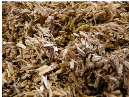
Fig. 2. Chemically modified hemp hurds used for composites preparing
