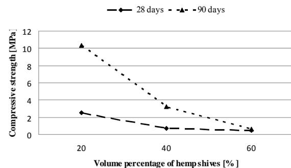
Fig. 2. Compressive strength of composites with different hemp hurds content (mixtures II.1-II.3) after 28 and 90 days of hardening
