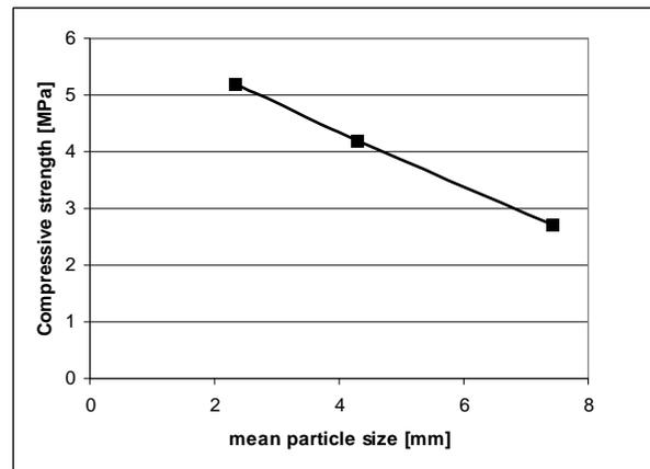
Fig. 4. Dependence of compressive strength on mean particle size of hemp hurds
