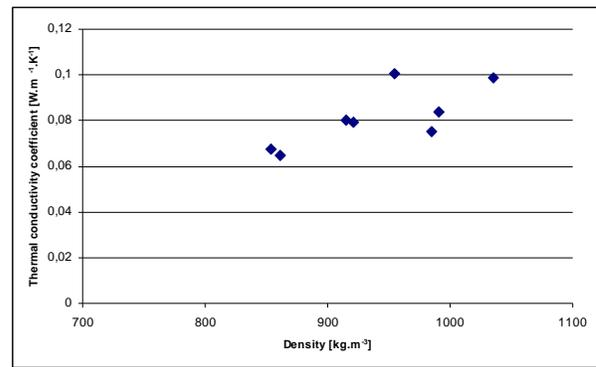
Fig. 8. Dependence of thermal conductivity coefficient on density of composites before and after thermal loading
