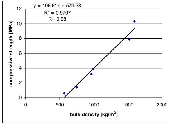
Fig. 3. Dependence of compressive strength on density for 90 days hardened composites
