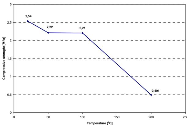
Fig. 5. Compressive strength of composites before and after thermal loading
