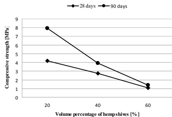
Fig. 1. Compressive strength of composites with different hemp hurds content (mixtures I.1-I.3) after 28 and 90 days of hardening
