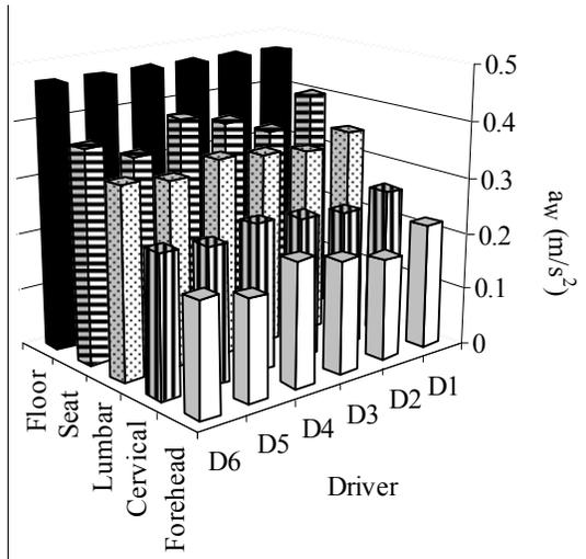
Fig. 3 Root mean square acceleration variation for 6 drivers (■) – floor, (≡) – seat, (⊘) – lumbar, (⊚) – cervical, (□) – forehead
