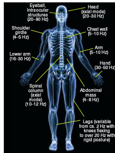
Fig. 1. Resonance frequencies of the human body
