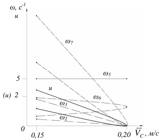
Fig.4. Graphs of angular velocities  $\omega_2$ ,  $\omega_3$ ,  $\omega_5$ ,  $\omega_6$ ,  $\omega_7$  and transmission ratio of mechanism ( $u$ ) in dependence of velocity of the center of rotation of driven link ( $\bar{V}_C$ )
