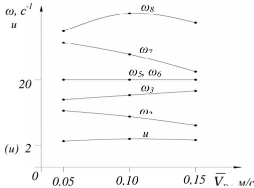
Fig.2. Graphs of angular velocities  $\omega_2, \omega_3, \omega_5, \omega_6, \omega_7, \omega_8$  and transmission ratio of mechanism ( $u$ ) in dependence of velocity of the center of rotation of driven link ( $\overline{V_D}$ )
