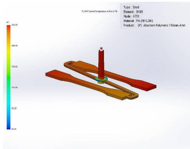
Fig. 6. The central temperature at the end of filling
