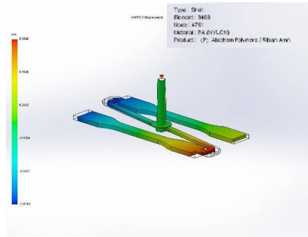
Fig. 20. Displacement in the Z direction
