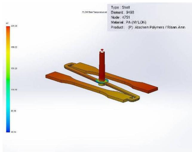
Fig. 8. The temperature of the melt volume
