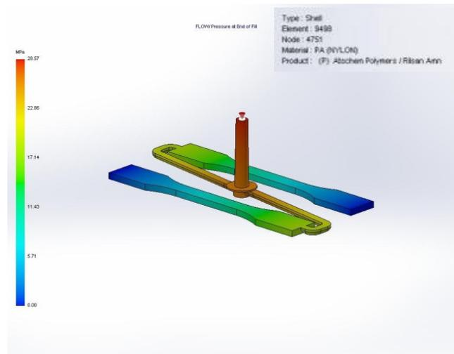
Fig. 5. The end of injection pressure
