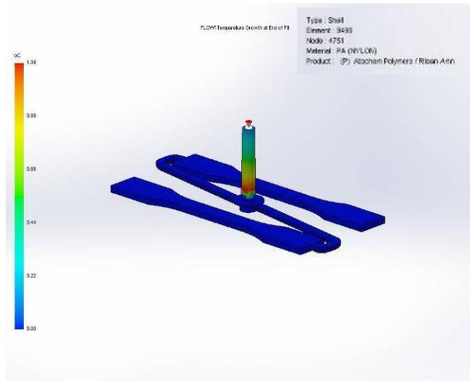
Fig. 11. The rise of temperature after filling
