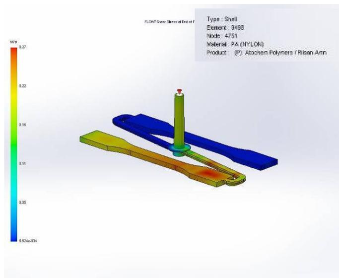
Fig. 12. The shearing tension
