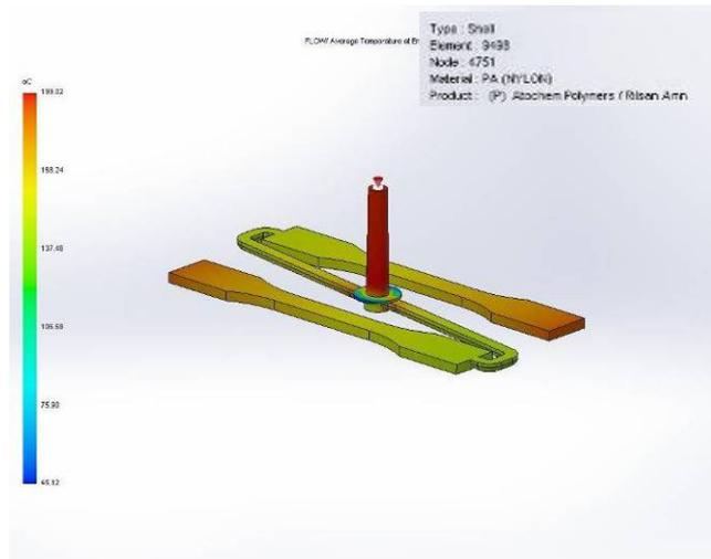
Fig. 7. The average temperature of the melt
