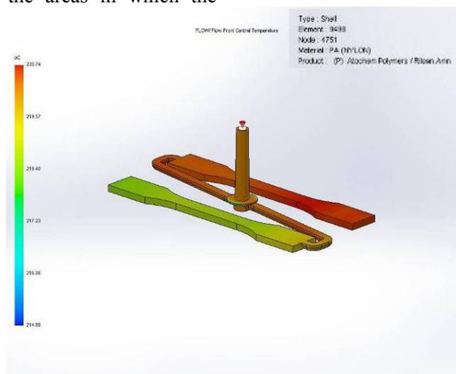
Fig. 9. Melt flow temperature
