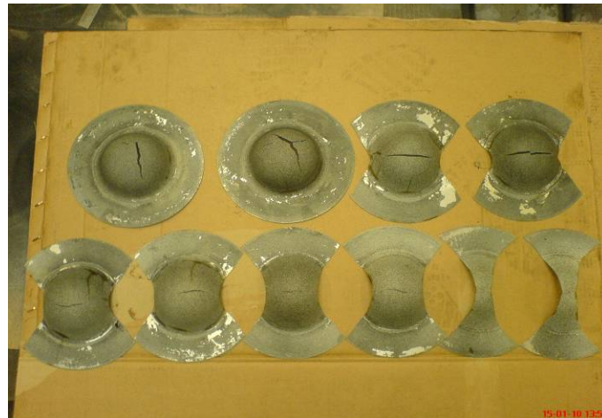
Fig.1. Deformed shapes of arc-shaped specimens obtained from the punch-stretch test.
