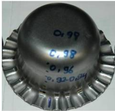
b) Fig. 7. a) Autoform solution of wall thinning values for BHF=17 kN b) Drawn cup and comparable thickness distribution of the cup wall for BHF=17 kN
