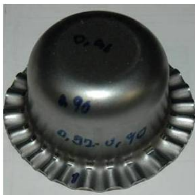
b) Fig. 8. a) Autoform solution of wall thinning values for BHF=23 kN b) Drawn cup and comparable thickness distribution of the cup wall for BHF=23 kN
