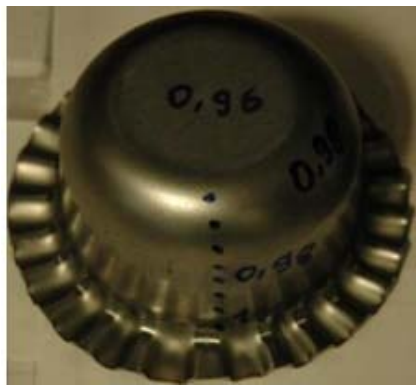
Fig. 6. a) Autoform solution of wall thinning values for BHF=12.5 kN b) Drawn cup and comparable thickness distribution of the cup wall for BHF=12.5 kN
