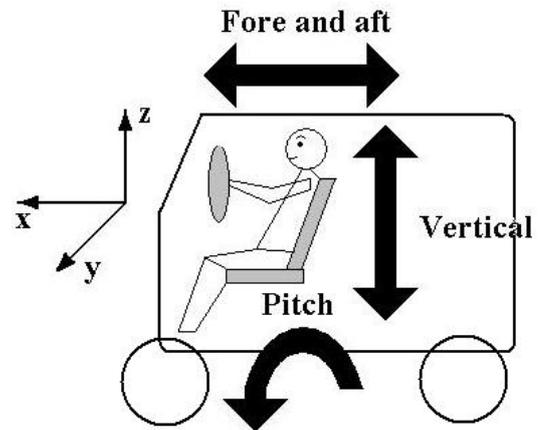
Fig. 1. Directions of vibration
