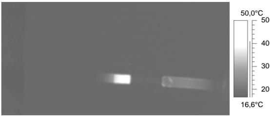
Fig.4. IR image of temperature field on the external, side surface of the pyrographite (PG) tube after its heating for 60.38 seconds by immobile copper rod of temp. ca. 50°C partly inserted into the PG tube.
