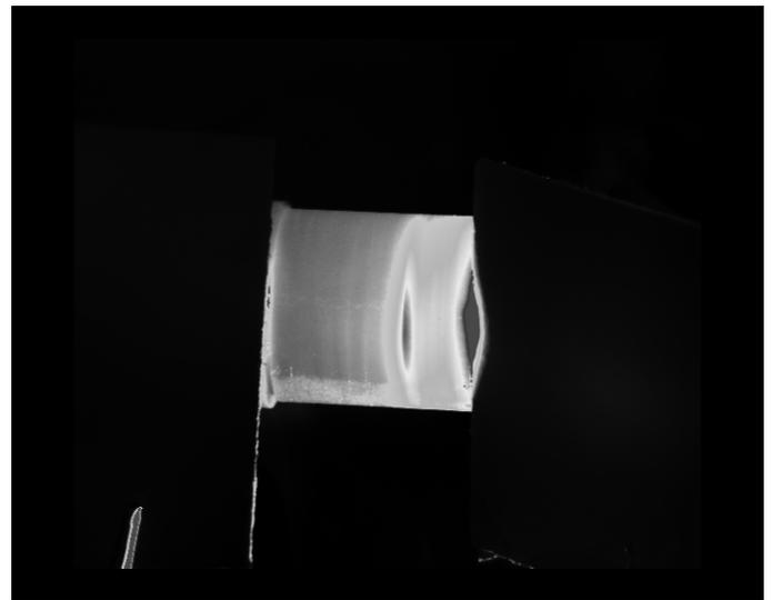
Fig.7. IR image of curved heat front moving on the external, side surface of pyrographite (PG) stack at the beginning of hot liquid flow through the open (from both ends) eccentric, narrow conduit drilled in the (PG) stack.
