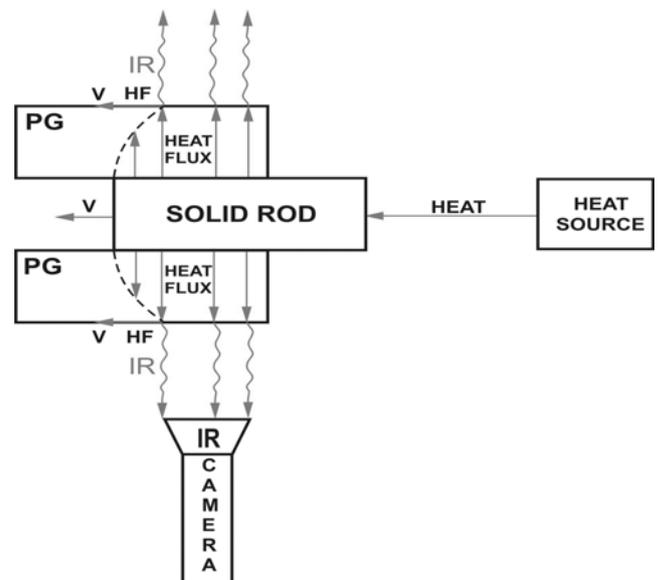
Fig.2. Schematic diagram of experimental set-up measuring by IR camera temperature field evolution on the external, side surface of the pyrographite (PG) tube, induced by moving with  $V$  velocity solid rod inserted into the PG tube and heated by external heat source; HF-heat front moving with  $V$  velocity on the external, side surface of the PG tube, along its axis.
