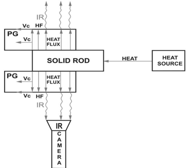
Fig.1. Schematic diagram of experimental set-up measuring by IR camera temperature field evolution on the external, side surface of the pyrographite (PG) tube, induced by the immobile solid rod inserted into the PG tube and heated by external heat source; HF-heat front (directly generated by hot immobile solid rod) moving in the PG tube wall with  $V_c$  velocity along the PG tube axis.
