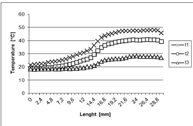
Fig.6. Measured by IR camera evolution of temperature distribution along external, side surface of the pyrographite (PG) tube after its heating for  $t_1 = 124.88$  s,  $t_2 = 60.38$  s,  $t_3 = 25.35$  s periods by immobile copper rod of temp. ca. 50°C partly inserted into the PG tube.
