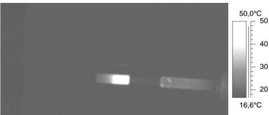
Fig.5. IR image of temperature field on the external, side surface of the pyrographite (PG) tube after its heating for 124.88 seconds by immobile copper rod of temp. ca. 50°C partly inserted into the PG tube.
