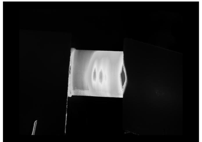
Fig.8. IR image of curved heat front moving on the external side surface of pyrographite (PG) stack during later stage of hot liquid flow through the open (from both ends) eccentric, narrow conduit drilled in the (PG) stack.
