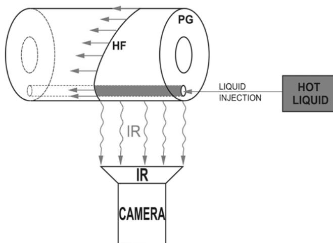
Fig.3. Schematic diagram of experimental set-up measuring by IR camera temperature field evolution on the external, side surface of the pyrographite (PG) stack of rings, induced by movement of hot liquid flowing through the open in both ends, narrow, eccentric conduit made in the PG stack, parallel to its longitudinal axis; HF- Curved heat front/zone moving on the external, side surface of pyrolytic graphite stack with the same velocity as head of hot liquid stream in the eccentric conduit.
