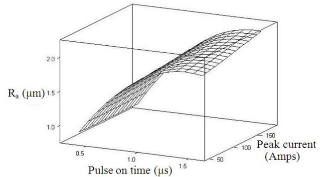
Fig. 4. Effect of pulse on time and peak current on  $R_a$  for fixed pulse frequency of 51.95 KHz and Job thickness of 13mm
