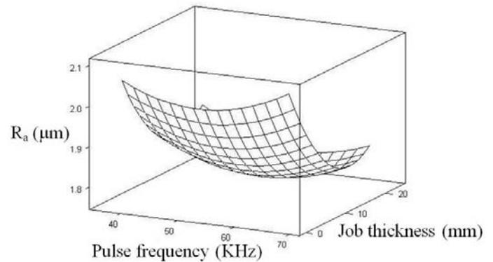
Fig. 5. Effect of pulse frequency and Job thickness on  $R_a$  for fixed pulse on time of  $0.95\mu\text{s}$  and peak current of 120 Amps
