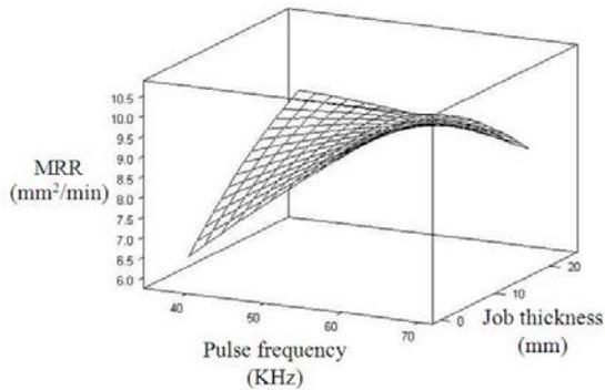
Fig. 3. Effect of pulse frequency and Job thickness on MRR for fixed pulse on time of  $0.95\mu\text{s}$  and peak current of 120 Amps
