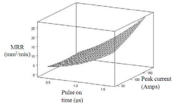
Fig. 2. Effect of pulse on time and peak current on MRR for fixed pulse frequency of 51.95 KHz and Job thickness of 13mm
