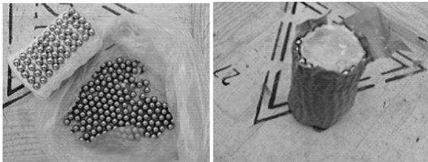
Fig. 1. Cylindrical explosive configuration
