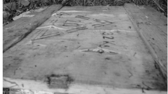
Fig. 3. Propulsion effects behind water screen with 10cm thickness
