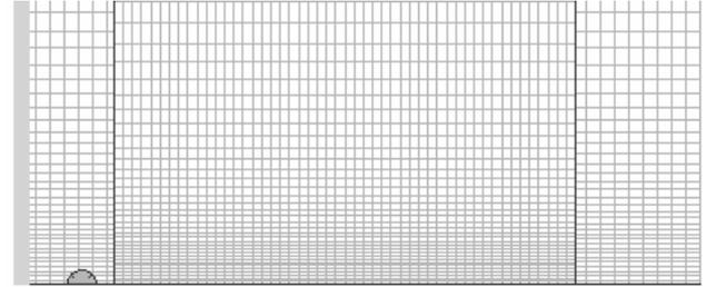
Fig. 6. Part of the rectangular mesh with lower grade zoning in J-direction
