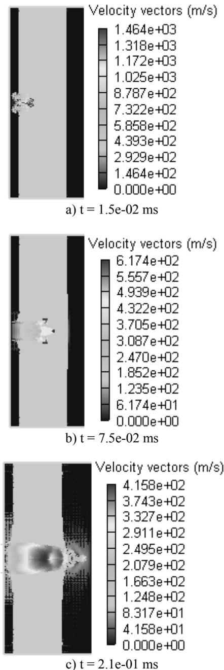
Fig. 8. Ball penetration on water layer with 100 mm thickness
