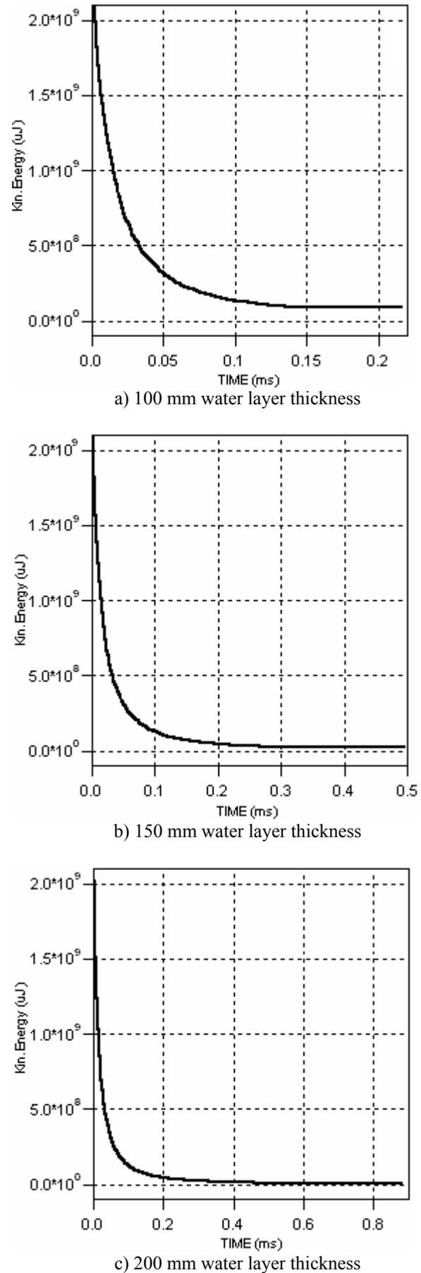
Fig. 9. Variation of the kinetic energy with time depending on water layer thickness
