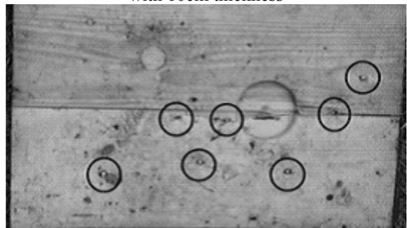
Fig.4. Propulsion effects behind water screen with 15 cm thickness
