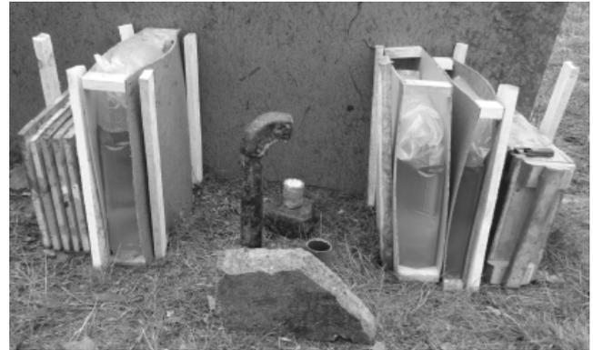
Fig. 2. Arrangement of water screens and explosive configuration on the first experiment
