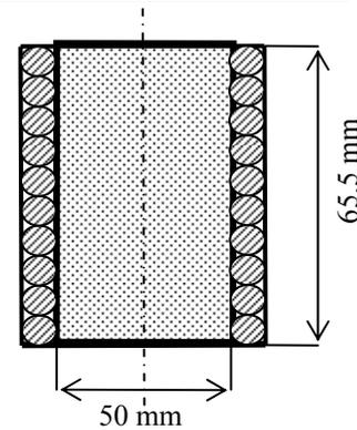
Fig. 5. Characteristics of explosive configuration
