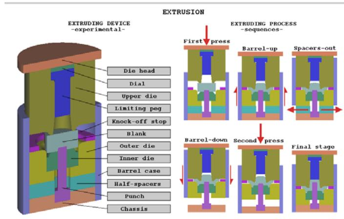
Fig. 14. Extruding tools and devices of the new technology
