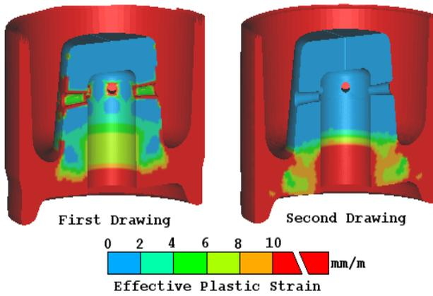
Fig. 11. Plastic strain after drawing operations
