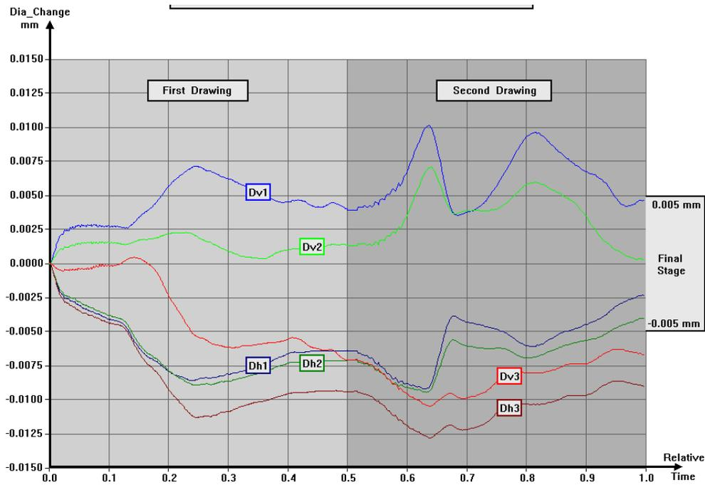
Fig. 12. Control diameters change in metal forming process
