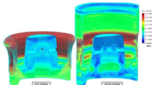
Fig. 10. Effective stress field simulated
