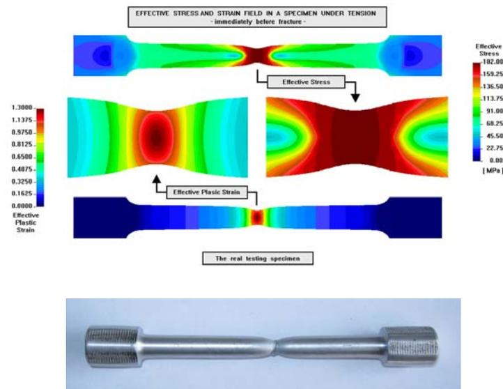
Fig. 7. Effective stress and strains field
