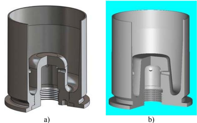
Fig. 1. Two pressure chambers (TPC) cartridge cases
