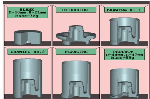
Fig. 2. Metal forming process
