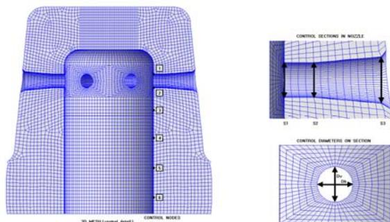
Fig. 9. Solid 3D mesh - details
