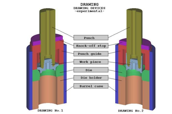
Fig. 15. Drawing device
