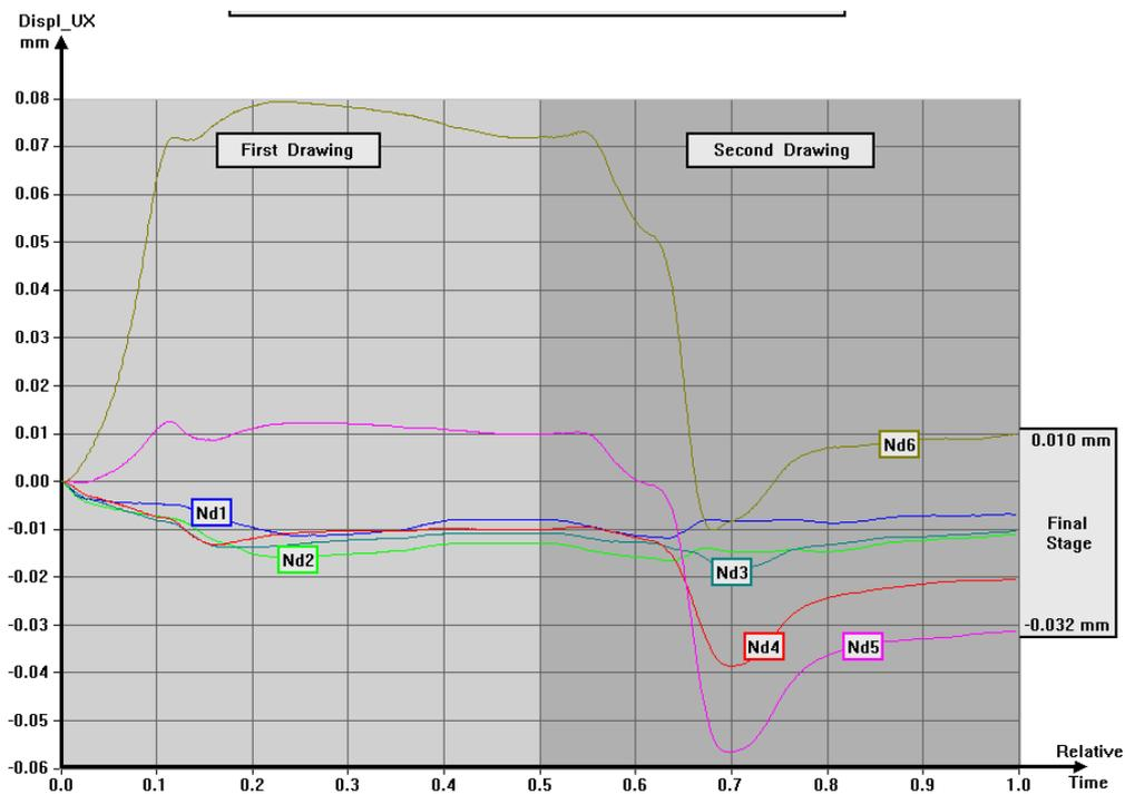
Fig. 13. Control nodes displacement in metal forming process
