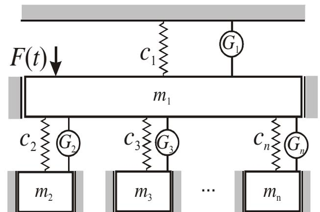
Fig.7. The model of a discrete mechanical system with active components
