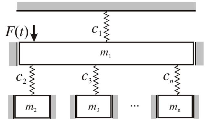
Fig.3. The example model of a restrained system obtained after decomposition of a characteristic function expressed in the form of slowness into a partial fractions with excitations.
