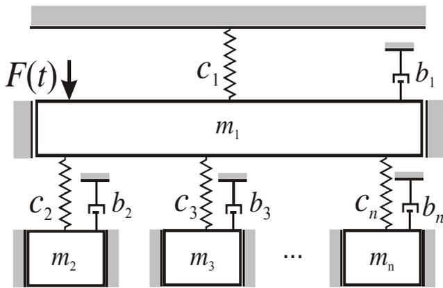
Fig.5. The model for a discrete mechanical system with passive components proportional to inertial components
