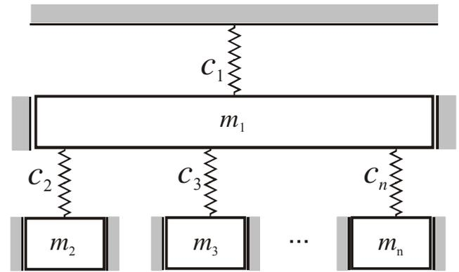
Fig.2. The example model of a restrained system obtained after decomposition of a characteristic function expressed in the form of slowness into a partial fractions.
