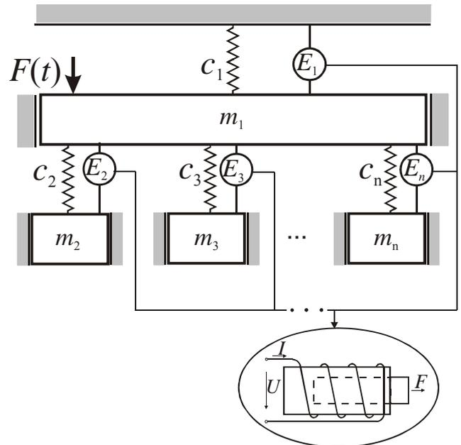
Fig. 9. A model of the system with electric elements – coil with moving core
