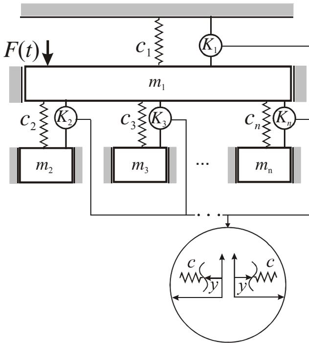
Fig. 8. A model of the system with kinematic excitations
