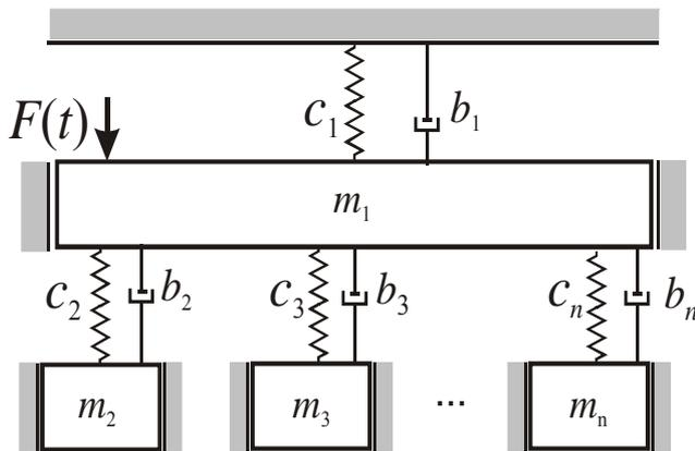
Fig.6. The model for a discrete mechanical system with passive components proportional to elastic components
