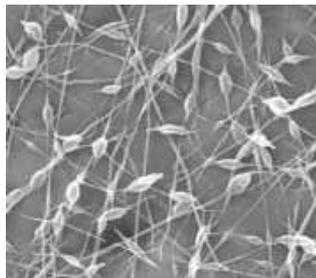
Fig. 8. Fibers with beads from PEO/chloroform solution electrospinning
