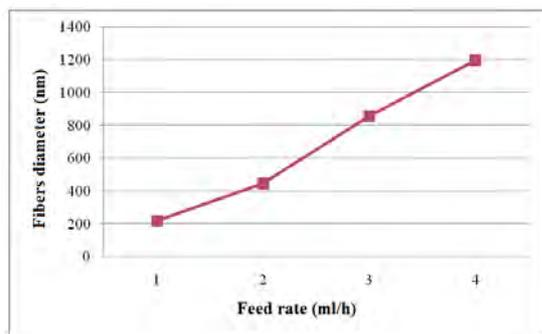
Fig. 15. Influence of the feeding rate on the fiber diameter ( $Q_1=1\text{ml/h}$ ,  $Q_2=2\text{ml/h}$ ,  $Q_3=3\text{ml/h}$ ,  $Q_4=4\text{ml/h}$ ,  $V=12\text{kV}$ ,  $d=60\text{cm}$ , syringe diameter= $10\text{ mm}$ , syringe volume= $3\text{ ml}$ , needle inner diameter= $0.7\text{ mm}$ ), [7]
