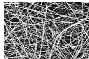
Fig. 6. SEM image of the PEO/ethanol nanofibers
