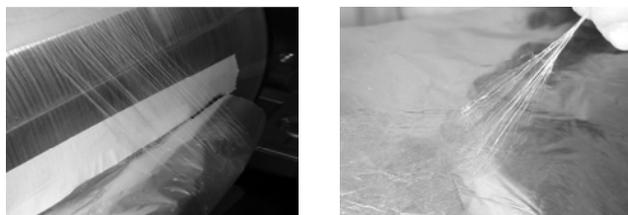
Fig. 4. Image presenting PEO/chloroform nanofibers when detaching from the rotary drum
