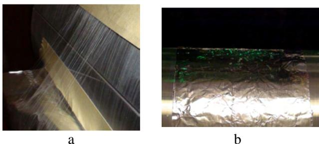
Fig. 12. a. Fibers detached from the collector; b. Drops deposited on the collector ( $Q=1\text{ml/h}$ ,  $V=10\text{kV}$ ,  $d=60\text{cm}$ , syringe diameter=10 mm, syringe volume= 3 ml, needle inner diameter=0,7 mm)
