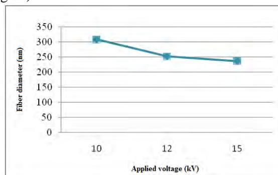
Fig. 13. Influence of the applied voltage upon the fiber diameter ( $Q=1\text{ml/h}$ ,  $V_1=10\text{kV}$ ,  $V_2=12\text{kV}$ ,  $V_3=15\text{kV}$ ,  $d=60\text{cm}$ , syringe diameter=10 mm, syringe volume= 3 ml, needle inner diameter=0.7 mm)
