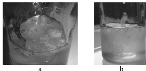
Fig. 2. 3% PEO/chloroform solution: a. sample taken immediately after the stirring of the polymer with the solvent; b. sample taken at 6 hours after dissolution
