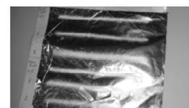
Fig. 7. Nanofibers deposited on the aluminium foil taken from the plane collector
