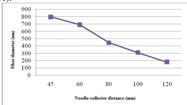
Fig. 11. Influence of the needle – collector distance upon the fiber diameter ( $Q=1\text{ml/h}$ ,  $V=10\text{kV}$ ,  $d_1=45\text{cm}$ ,  $d_2=60\text{cm}$ ,  $d_3=80\text{cm}$ ,  $d_4=100\text{cm}$ ,  $d_5=120\text{cm}$ , syringe diameter=10 mm, syringe volume= 3 ml, needle inner diameter=0.7 mm)
