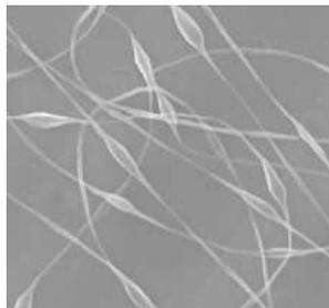
Fig. 9. Fibers with beads from PEO/ethanol solution electrospinning
