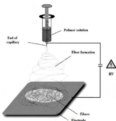
Fig. 1. The general basic diagram of the electrospinning process
