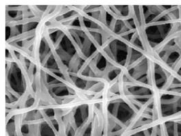
Fig. 5. SEM image of the PEO/chloroform nanofibers
