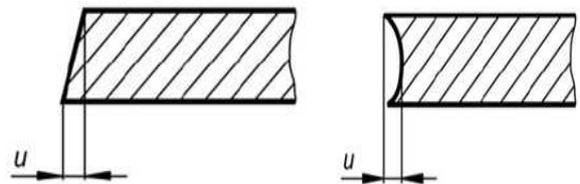
Fig. 4 Deviation from perpendicularity, [5]
