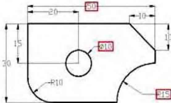
Fig. 6. Shape of the water jet processed piece
