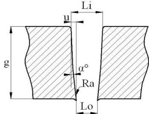
Fig. 3 The components of the surfaced processed with water jet with abrasive mixture, [4]
